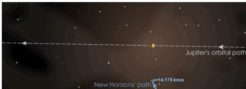
Figure 2. As you can see in this rough simulation, the New Horizons spacecraft's motion is at an angle to Jupiter's orbit as it approaches the July, 2007 flyby. Notice the speed of the spacecraft is about 14 km/s.
