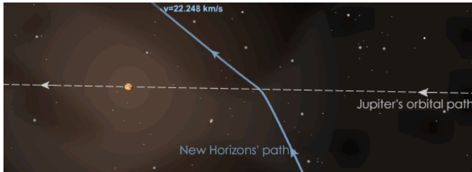
Figure 3. As the New Horizons spacecraft flew past Jupiter, which is traveling from right to left in this image, the spacecraft was pulled toward Jupiter by the planet's gravity. You can see that the path and the speed of the spacecraft were changed by the encounter.
