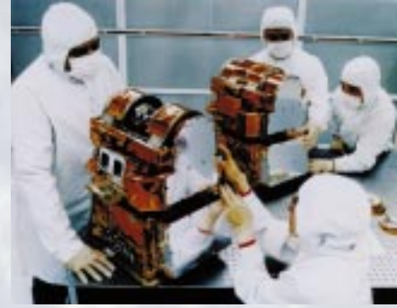
CERES instrument assembly (TRW)
