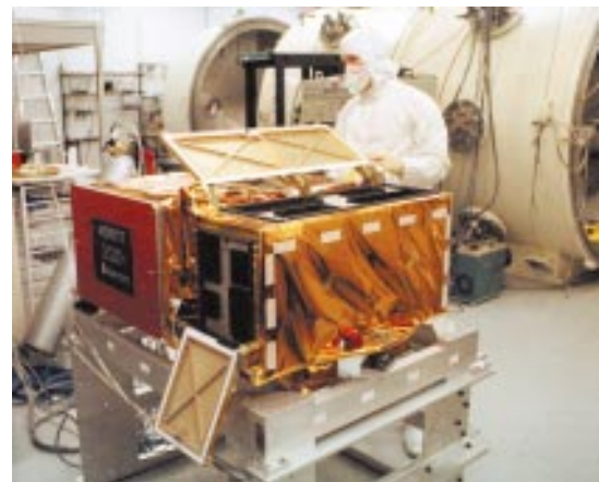
A COM DEV technician prepares the MOPITT instrument for flight
