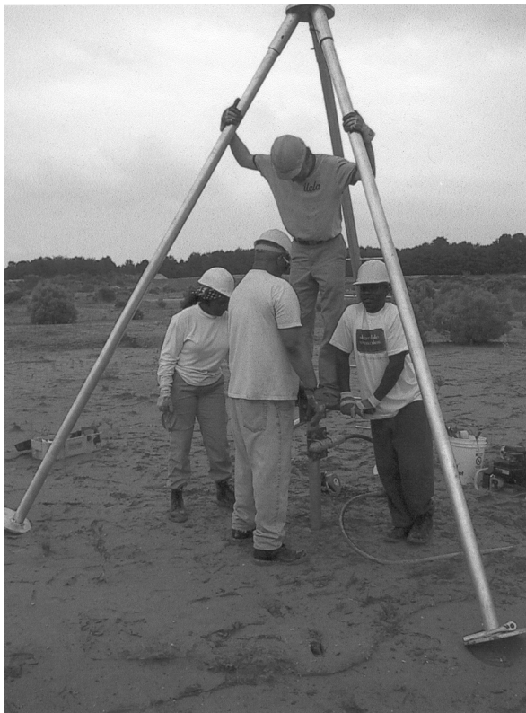
Figure 1. Author and teacher-students obtaining a continuous sediment core using a vibracoring apparatus.
