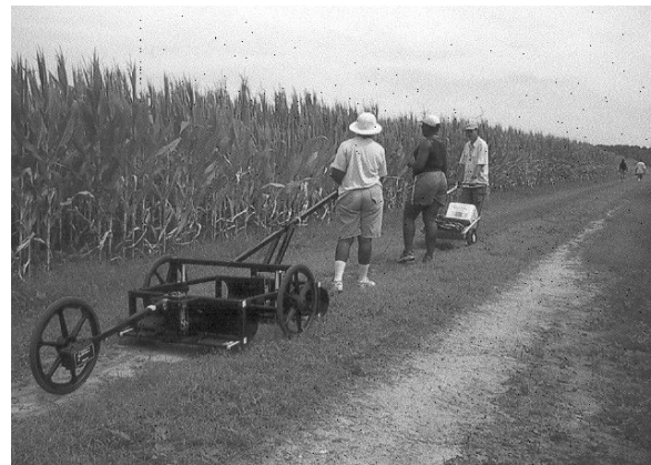
Figure 4. A geophysics team of teacher/researchers and author perform a common-offset profile using a ground penetrating radar (GPR) system.
