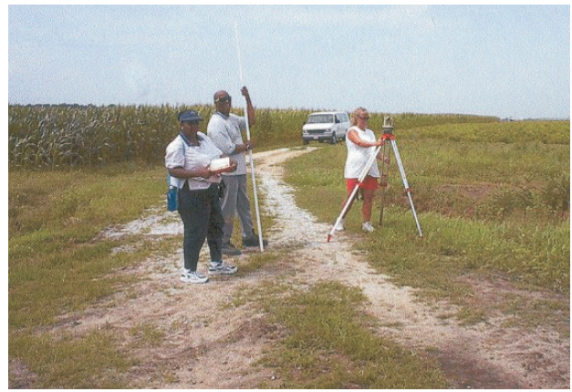
Figure 2. Students setting up a surveyor's transit for research site mapping and topographic profiling.
