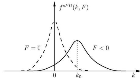
FIG. 3. Shifted distribution function. The dashed line corresponds to an equilibrium zero field case. The displayed wave vector  $k$  in the direction of the field has a shift  $k_0$  proportional to average drift velocity of electrons. The other, perpendicular direction is not shifted, but the broadening (described by the increased electron temperature) is present in either direction.
