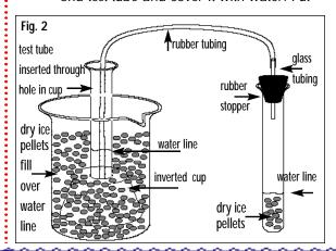
the stopper into the test tube and attach the rubber tubing to the glass tubing in the test tube stopper.
