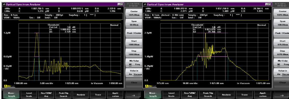
Figure 3-4 Examples of the laser output spectra under high (left) and low (right) pump intensity.
