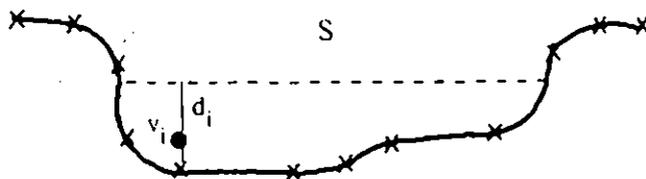
**Figure 2.3** Calibration data necessary for velocity predictions in IFG4
