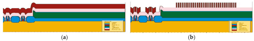
Figure 4. Photoresist deposition and etch.
