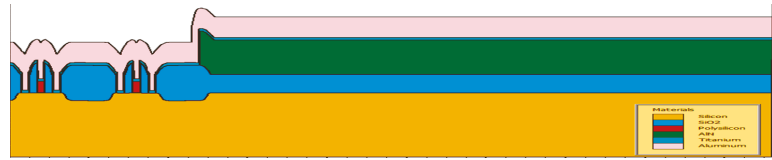
Figure 3. Metal layers deposition.
