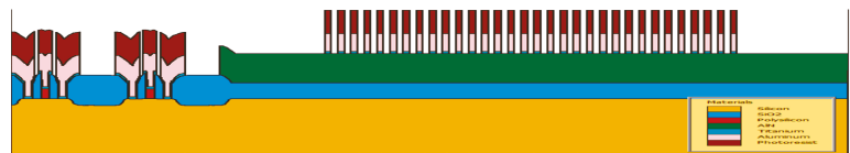
Figure 5. Titanium and aluminum etch.
