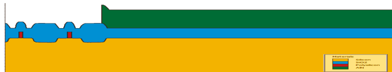
Figure 2. AlN piezoelectric layer deposition.
