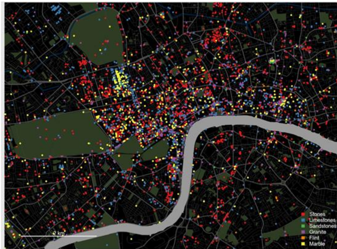
Figure 2. Spatial distribution of common building stones in London including stones (nonspecific), limestone (Portland, Clipsham, Caen and Rag) sandstone (Reigate and others) granite, flint and marble. Portland stone is the most common of the specified varieties.
