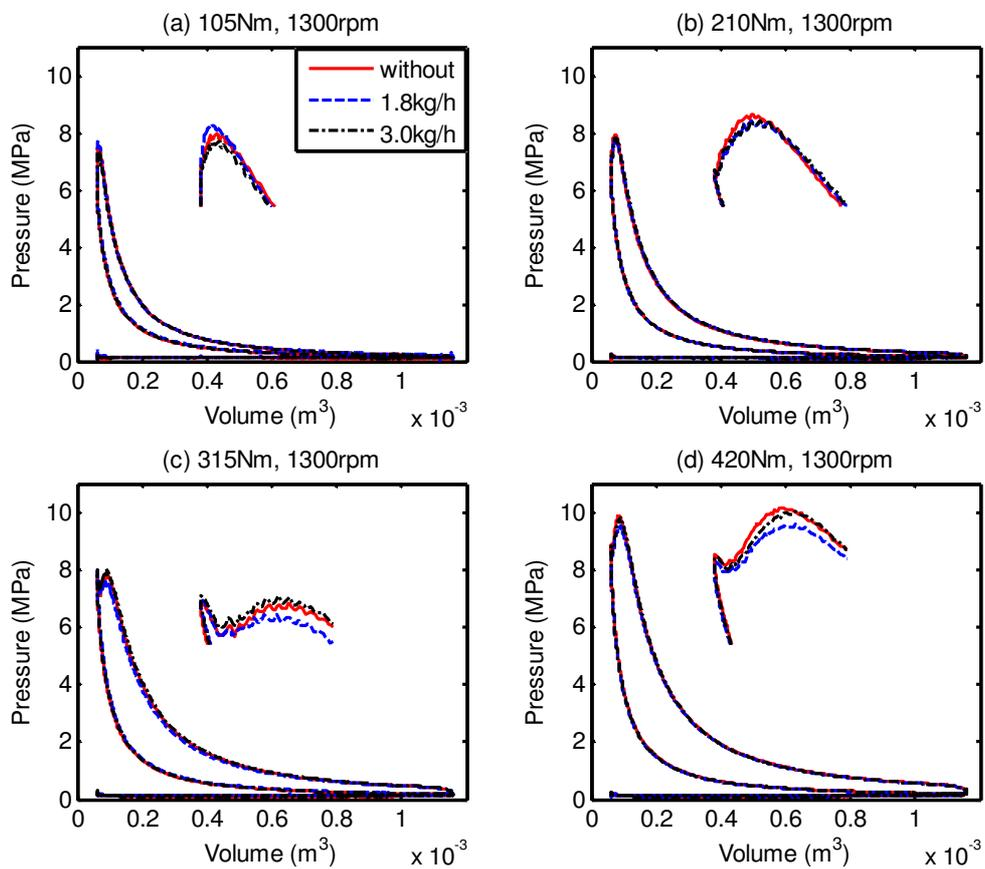
Figure 3 P-V diagram of CI engine at 1300rpm and various engine loads
