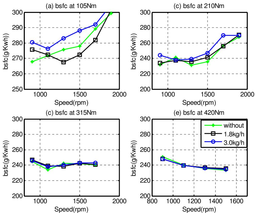
Figure 8 Brake specific fuel consumption (bsfc) at different loads
