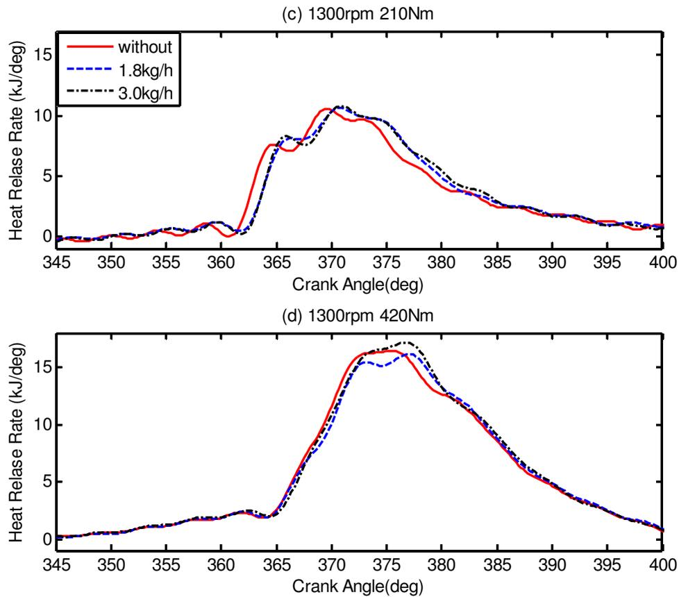
Figure 6 Heat releases rate at 1300rpm and different loads
