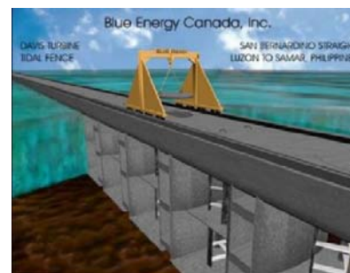
Figure 1.43. La structure "tidal bridge" ©[BEN-09]
