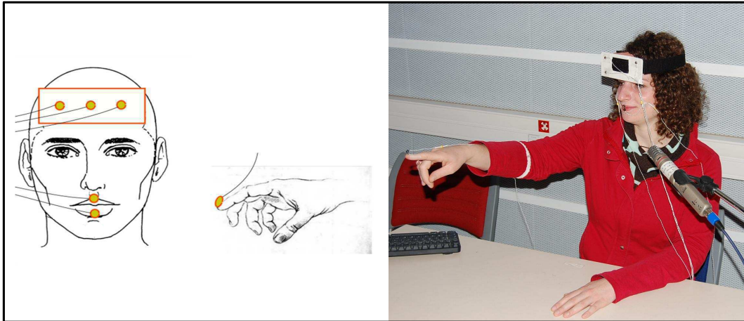
FIGURE 3.2 – Position des diodes émettrices infra-rouge (© C. Gonseth)
