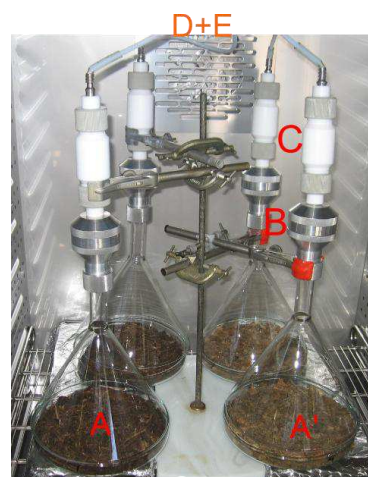
Fig. 1. Implementation of microcosms in a climatic chamber. A: organosoil, A': brownsoil, C: quartz filter holder, D: PUF holder, E: to the external KNF Laboport pump equipped with a Teflon membrane (5L/min).
