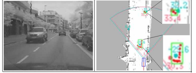
Fig. 8. Moving objects detected from laser data are confirmed by radar data.
