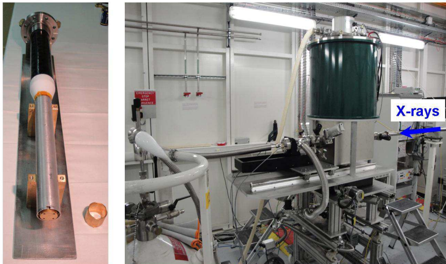
Figure 2.7 Probe (left) and the fridge with the X-rays line (right) used at the ID12 line at ESRF.
