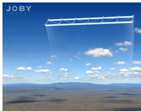
Figure I.11: Airborne wind turbines Imagined by Joby energy
