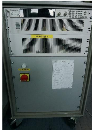
Figure 7.3 Controllable DC source
