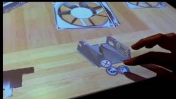
Finger tap on the object in individual space and access to the Menu for duplication, delete and annotation
