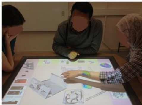
Figure 5-9: The first prototype of MT-DT testing rotation, translation and link creation function
