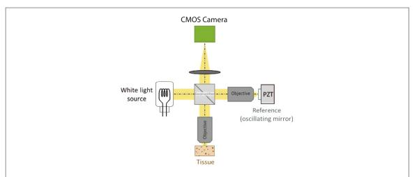
**Figure 1.** Optical layout of the full-field optical coherence tomography setup (FFOCT). As for standard OCT, the low coherence of the light source allows the sectioning of thin  $(0.8\,\mu\text{m})$  slices of diffusers inside thick biological tissues. Koehler illumination of the sample allows the parallel acquisition of around 1 million CMOS pixels, as in a standard wide-field microscope.
