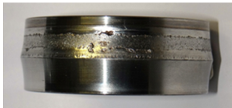
Figure 5: Flaking over the entire inner race of the faulty bearing.
