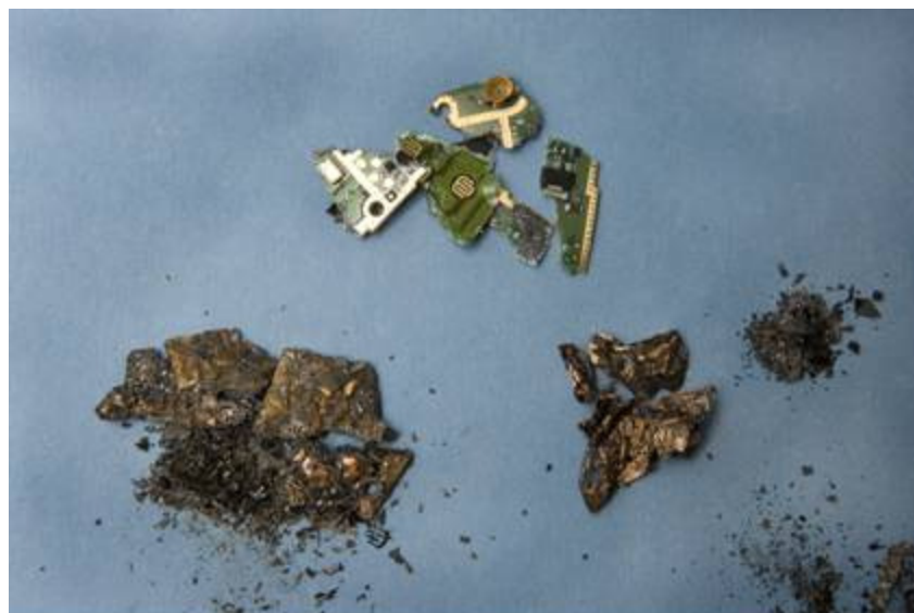
Figure 6 The effect of pyrolysis on printed circuit boards taken from mobile phones. The untreated boards (top centre) pyrolyse to form a friable residue (bottom left) that can easily be separated into the copper power boards and glass fibre (bottom right).
