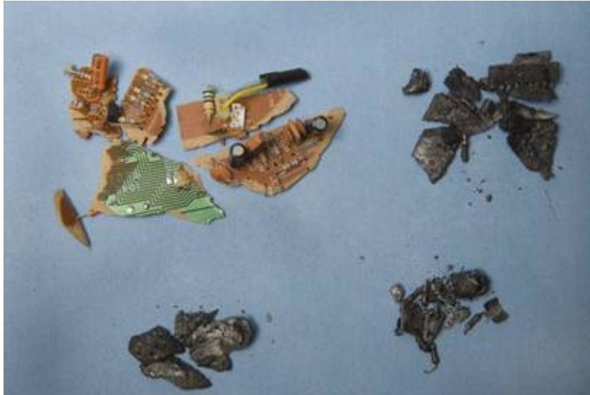
Figure 5 The effect of pyrolysis on printed circuit boards taken from televisions. The untreated boards (top left) pyrolyse to form a friable residue (top right) that can easily be separated into char (bottom left) and electrical components (bottom right).
