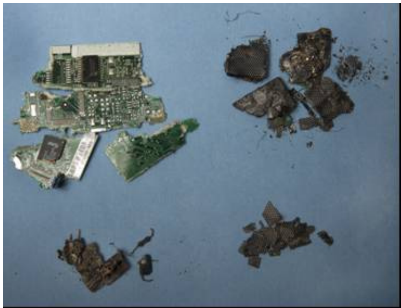
Figure 4 The effect of pyrolysis on printed circuit boards taken from computers. The untreated boards (top left) pyrolyse to form a friable residue (top right) that can easily be separated into the copper power boards and components (bottom left) and glass fibre (bottom right).
