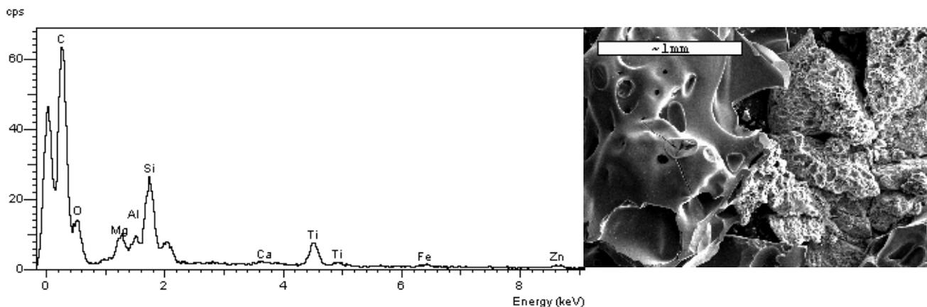
**Figure 7 SEM-EDX analysis of the mixed WEEE plastic pyrolysis char**
