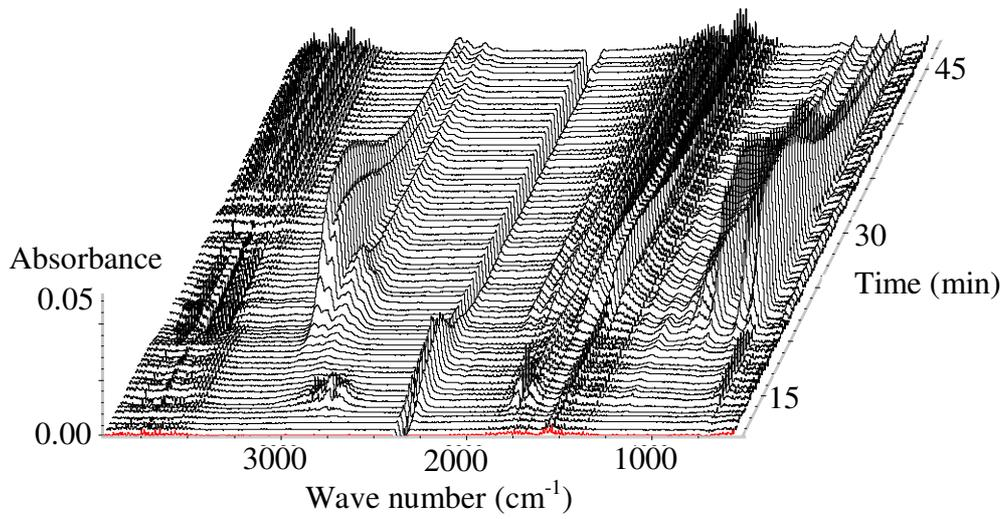
**Figure 3 TGA-FT-ir analysis of the Refrigeration plastic**
