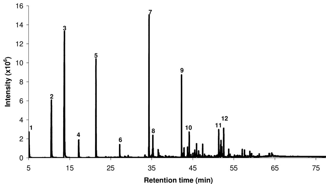
**Figure 12 GC-MS analysis of the oil resulting from the pyrolysis of the CRT plastic in a fixed bed reactor**
