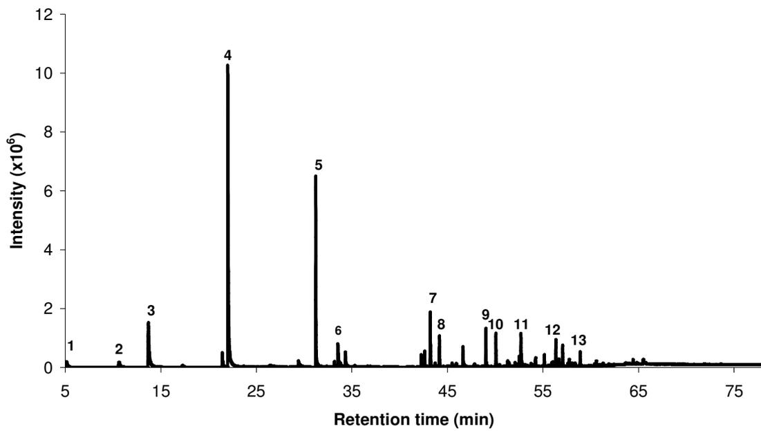
**Figure 14 GC-MS analysis of the oil resulting from the pyrolysis of the mixed WEEE plastic in a fixed bed reactor**
