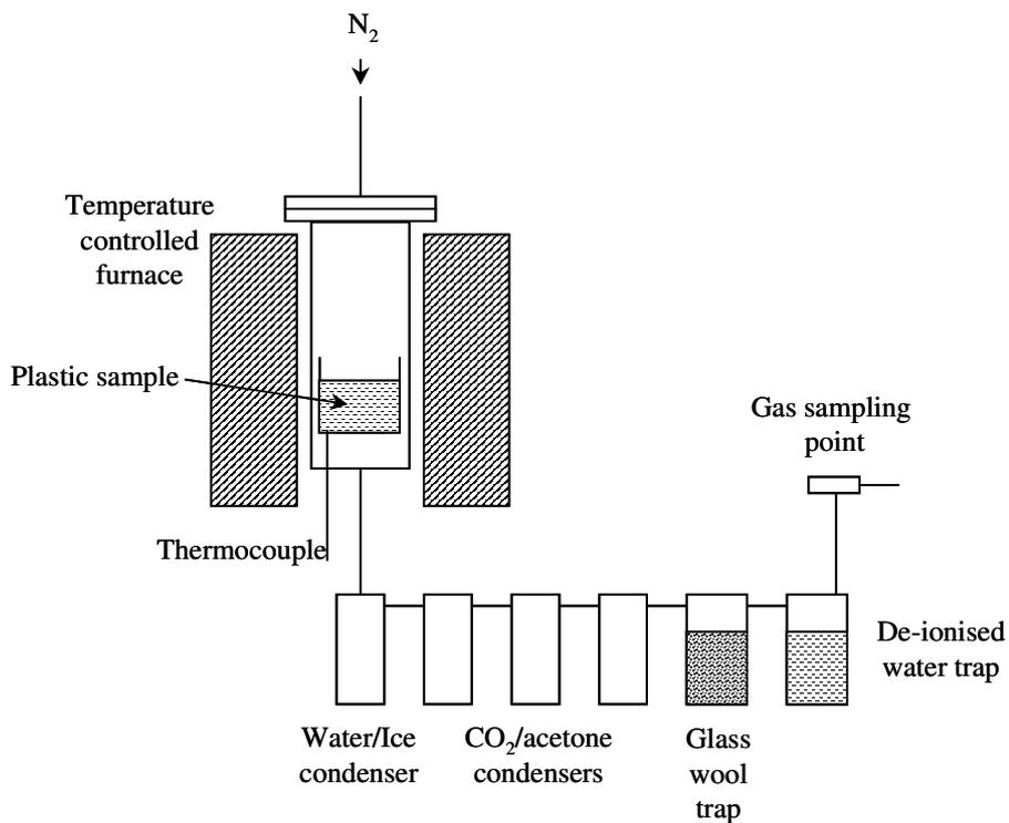
**Figure 1 Schematic of the fixed bed reactor**
