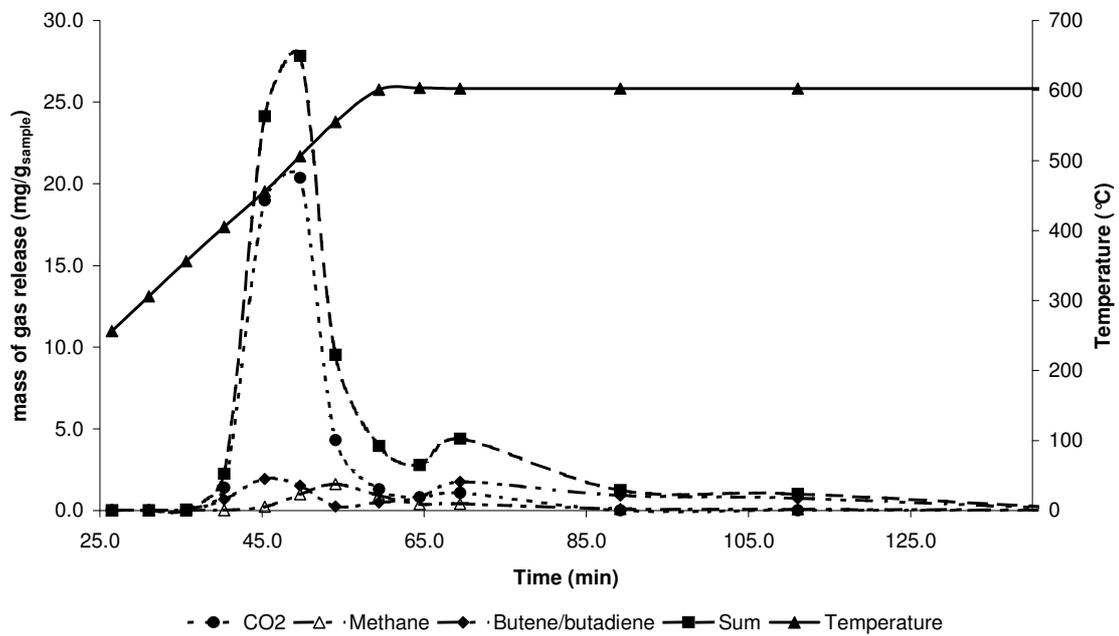
**Figure 10 Profile of the gases released during batch pyrolysis of the mixed WEEE plastic in a fixed bed reactor**
