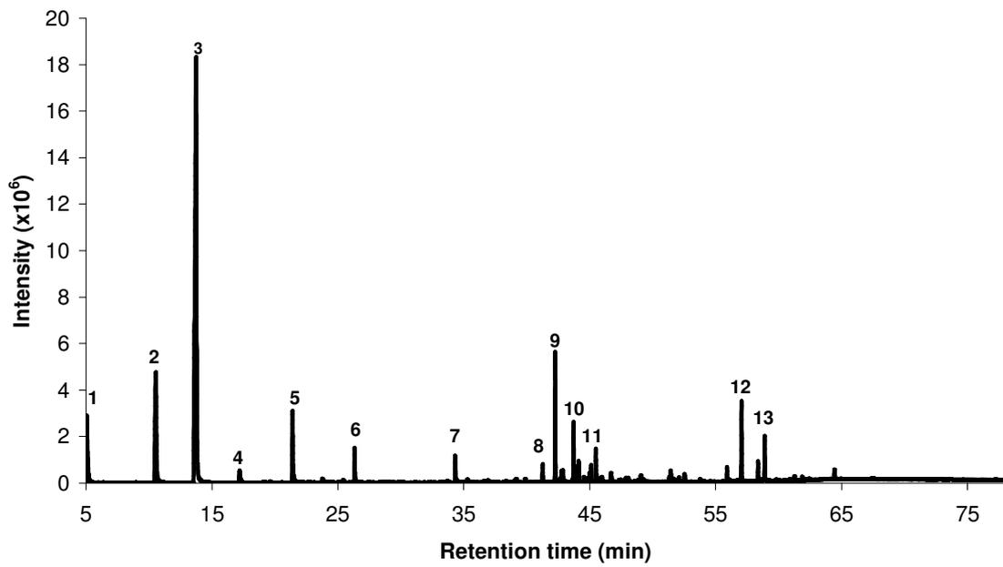
**Figure 13 GC-MS analysis of the oil resulting from the pyrolysis of the Refrigeration plastic in a fixed bed reactor**
