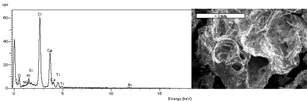
**Figure 6 SEM-EDX analysis of the Refrigeration plastic pyrolysis char**
