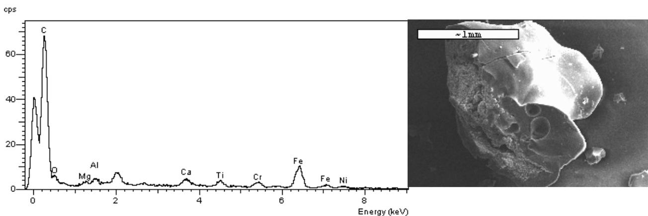
**Figure 5 SEM-EDX analysis of the CRT pyrolysis char**
