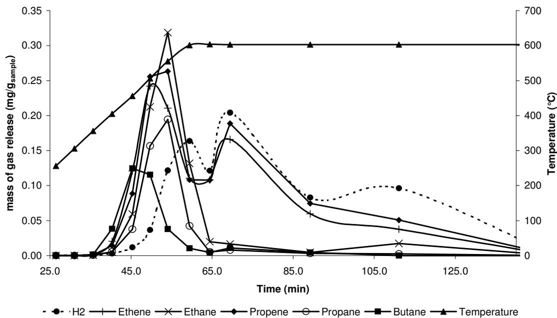
**Figure 11 Organic gases released during the batch pyrolysis of the mixed WEEE plastic in a fixed bed reactor**
