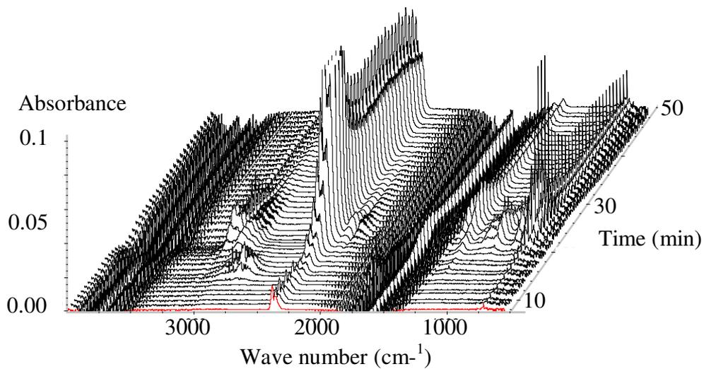
**Figure 4 TGA-FT-ir analysis of the mixed WEEE plastic**
