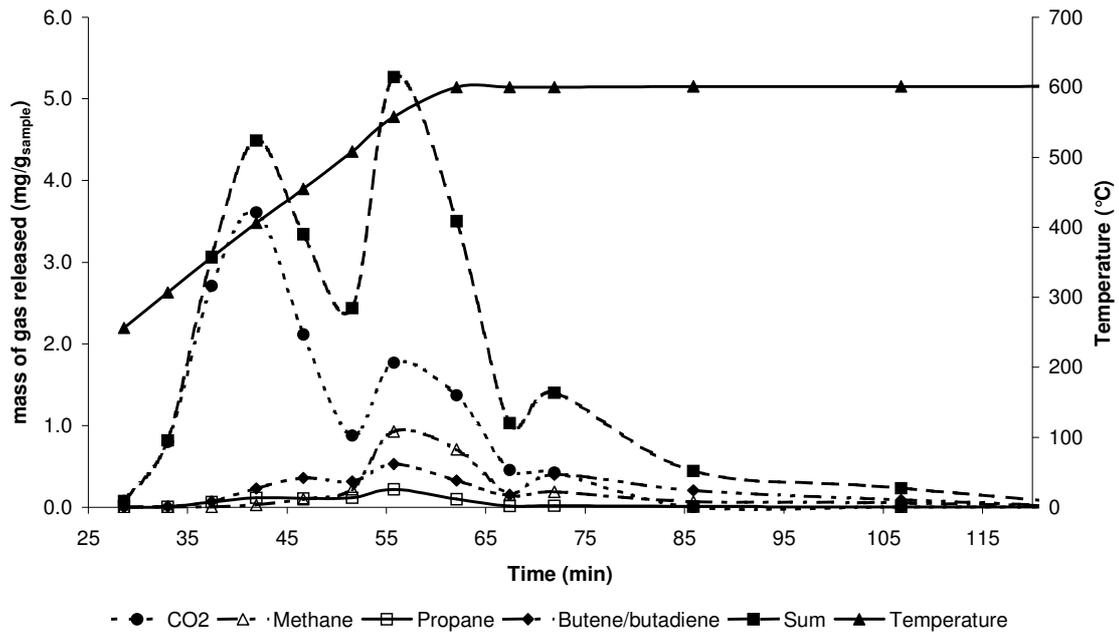
**Figure 9 Profile of the release of gases during batch pyrolysis of the refrigeration plastic in a fixed bed reactor**
