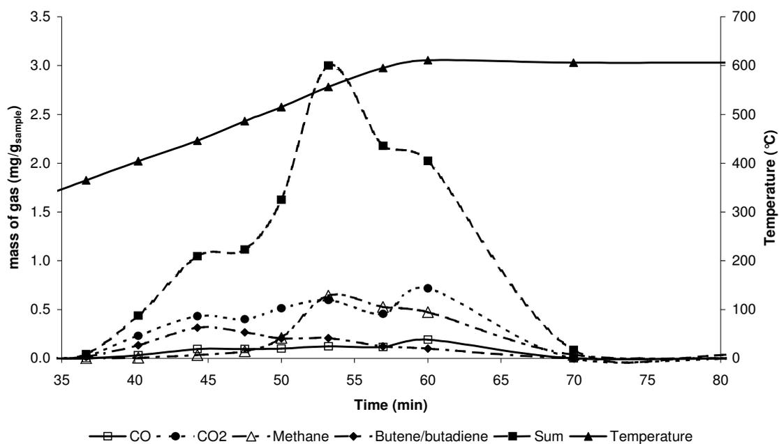
**Figure 8 Profile of the release of gases during the batch pyrolysis of CRT plastic in a fixed bed reactor**
