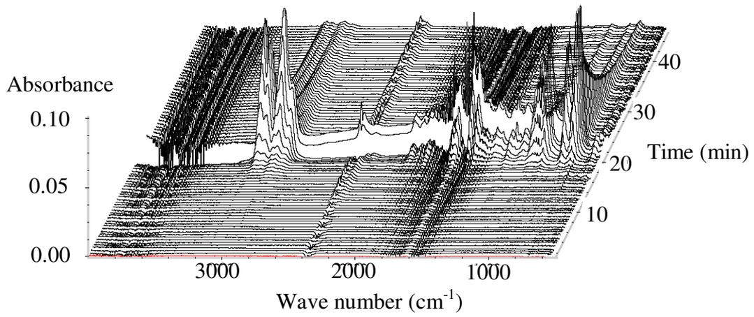
**Figure 2 TGA-FT-ir analysis of the CRT plastic**
