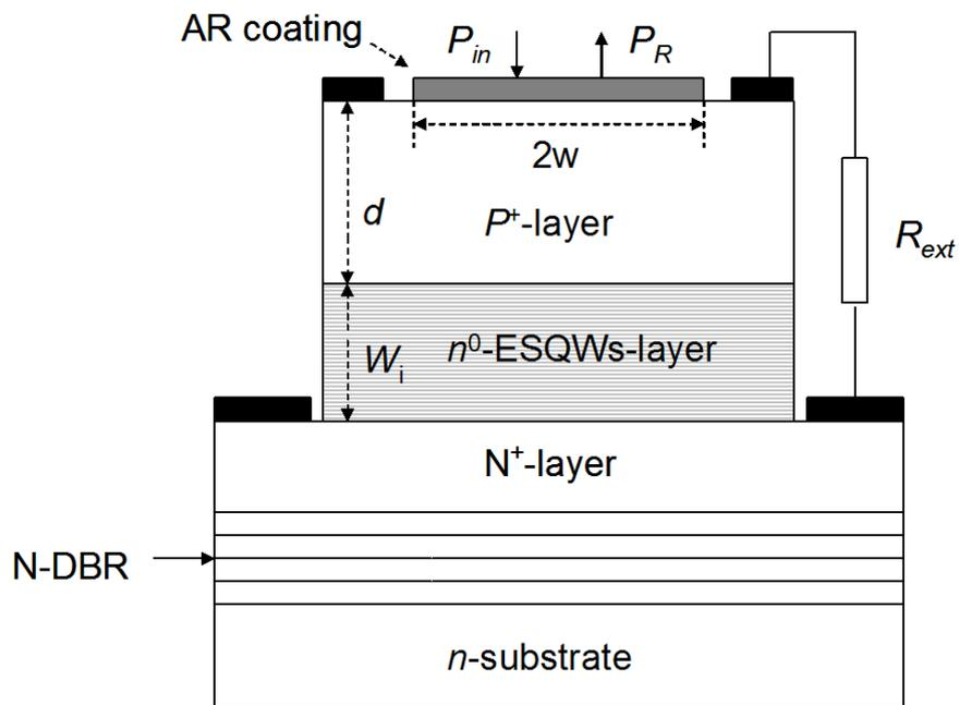
FIG. 1: Schematical view of a self-biased surface normal Extremely Shallow Quantum Well electroabsorptive self-biased SESAM.  $w$  is the radius of the light spot.
