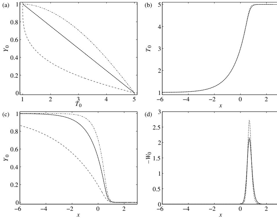
**Figure 1.** (a) Steady solutions in the  $(T_0, Y_0)$ -plane and spatial profiles of (b) temperature, (c) fuel mass fraction and (d) reaction rate, for  $Q = 4$ ,  $\theta = 70$  ( $\beta = 11.2$ ) and Lewis numbers 0.3 (dashed lines), 1.0 (solid lines) and 1.8 (dot-dashed lines). Also shown are the profiles for  $\theta = 90$  ( $\beta = 14.4$ ),  $Le = 1.0$  (dotted lines).
