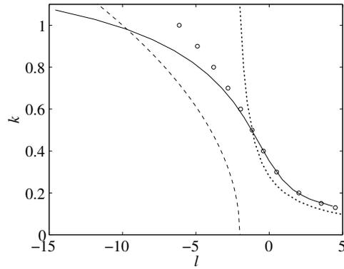
**Figure 2.** Neutral stability boundary in the  $(l, k)$ -plane for  $Pr = 0.75$ ,  $Q = 5$  and  $\theta = 70$  ( $\beta = 9.72$ ). Also shown are the infinite activation temperature results from Jackson & Kapila (1984) (open circles), the SVF results from Matalon & Matkowsky (1982) (dotted line) and the CDA results of Sivashinsky (1977) (dashed line).
