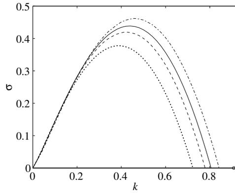
**Figure 6.** Dispersion relations for  $Pr = 0.75$ ,  $Q = 4$ ,  $l = -5$  and dotted line:  $\theta = 30$  ( $\beta = 4.8$ ,  $Le = 0.4898$ ), dashed line:  $\theta = 50$  ( $\beta = 8$ ,  $Le = 0.6154$ ), solid line:  $\theta = 70$  ( $\beta = 11.2$ ,  $Le = 0.6914$ ) and dot-dashed line  $\theta = 140$  ( $\beta = 22.4$ ,  $Le = 0.8175$ ). Also shown as an open circle is the infinite activation temperature neutrally stable wavenumber.
