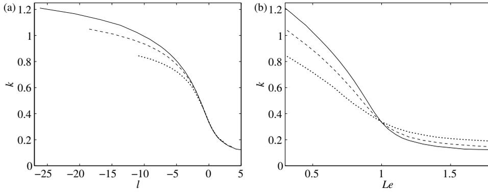
**Figure 4.** Neutral stability boundaries in (a) the  $(l, k)$ -plane and (b) the  $(Le, k)$ -plane, for  $Pr = 0.75$ ,  $Q = 4$  and dotted lines:  $\theta = 30$  ( $\beta = 4.8$ ), dashed lines:  $\theta = 50$  ( $\beta = 8$ ) and solid lines:  $\theta = 70$  ( $\beta = 11.2$ ).
