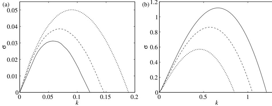
**Figure 5.** Dispersion relations for  $Pr = 0.75$ ,  $Q = 4$ , (a)  $Le = 1.8$  and (b)  $Le = 0.3$ , and dotted lines:  $\theta = 30$  ( $\beta = 4.8$ ), dashed lines:  $\theta = 50$  ( $\beta = 8$ ) and solid lines:  $\theta = 70$  ( $\beta = 11.2$ ).
