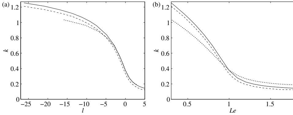
**Figure 7.** Neutral stability boundaries in (a) the  $(l, k)$ -plane and (b) the  $(Le, k)$ -plane, for  $Pr = 0.75$  and dotted lines:  $Q = 8, \theta = 70$  ( $\beta = 6.91$ ), dashed lines:  $Q = 4, \theta = 70$  ( $\beta = 11.2$ ) and solid line:  $Q = 8, \theta = 113.4$  ( $\beta = 11.2$ ).
