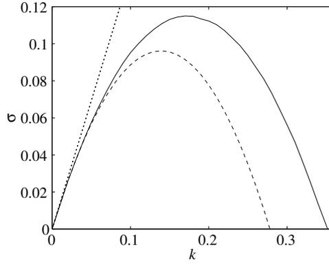
**Figure 3.** Dispersion relation for  $Pr = 0.75$ ,  $Q = 5$ ,  $Le = 1$  and  $\theta = 70$  ( $\beta = 9.72$ ). Also shown are the SVF (dashed line) and Landau-Darrieus (dotted line) dispersion relations.
