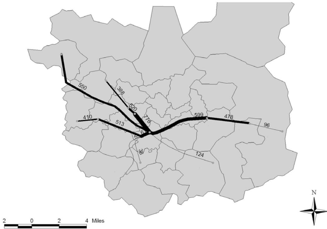
**Figure 8 : Assignment of rail passenger flows from urban stations to the centre of Leeds.**
