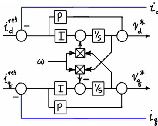
Figure 5.27 – Stationary regulator in synchronous frame.
