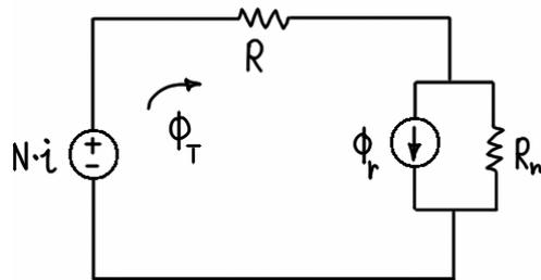
Figure 2.15 – Simplified magnetic circuit of Figure 2.12.
