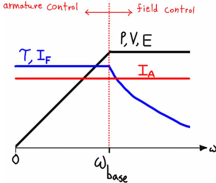
**Figure 5.20 – Maximum values for operation below and above base speed.**
