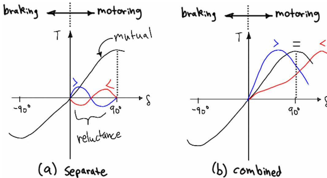
Figure 5.16 – Torque functions: (a) components; (b) combined.
