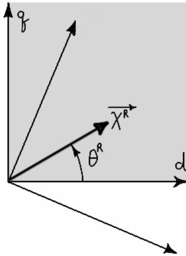
**Figure 3.38 – Park transform: rotor reference frame perspective.**
