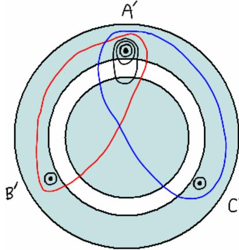
**Figure B.3 – One-half of the flux paths linking phase-A.**
