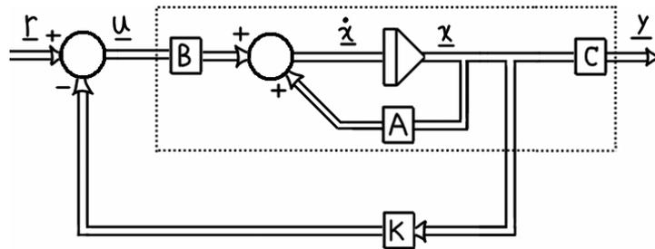
**Figure 6.5 – Full state feedback controller.**
