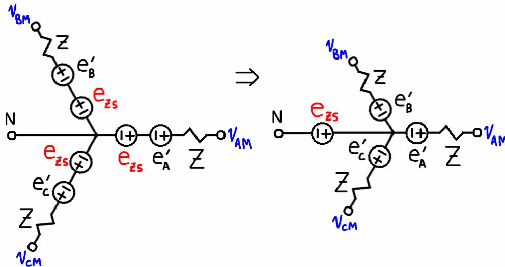
**Figure D.8 – Equivalent motor bEMF arrangement.**
