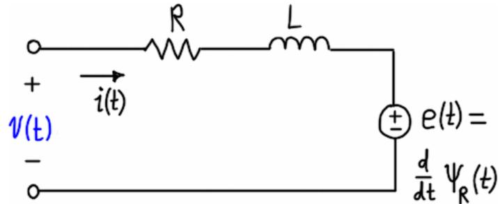
**Figure 2.18 – Per-phase electrical model of general brushless PM motor; explicit inductor.**
