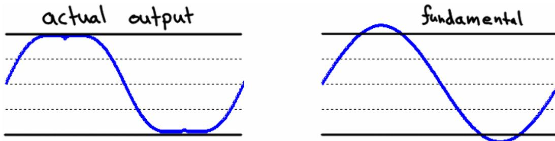
Figure 4.20 – Third harmonic injection can produce larger fundamental than SPWM.
