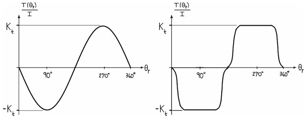
**Figure 2.22 – Torque functions of sinusoidal and arbitrary trapezoidal motors.**
