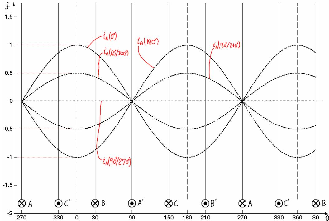
**Figure 3.5 – Stator MMF distribution of phase-A at various electrical positions in time.**
