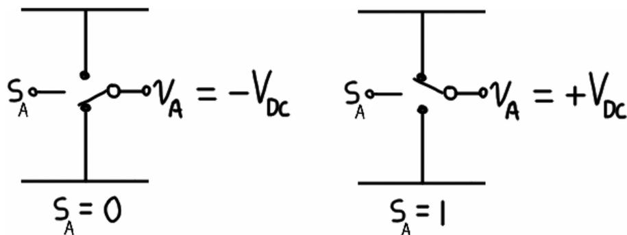
Figure 4.7 – Leg states for 180° inverter.
