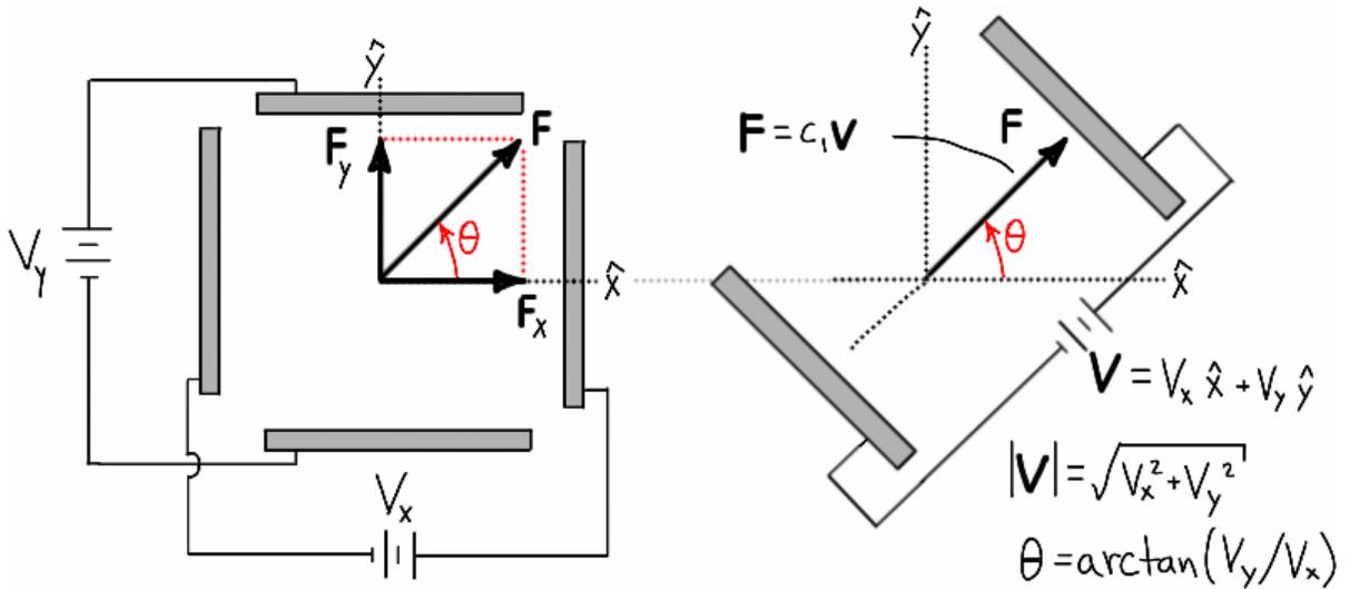
**Figure 3.24 – Equivalent force produced by plates aligned with resultant force.**
