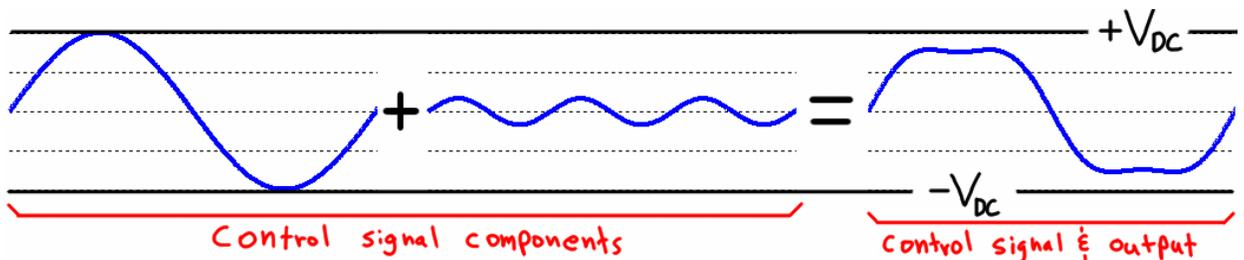
Figure 4.19 – Adding the third harmonic reduces peak amplitude.
