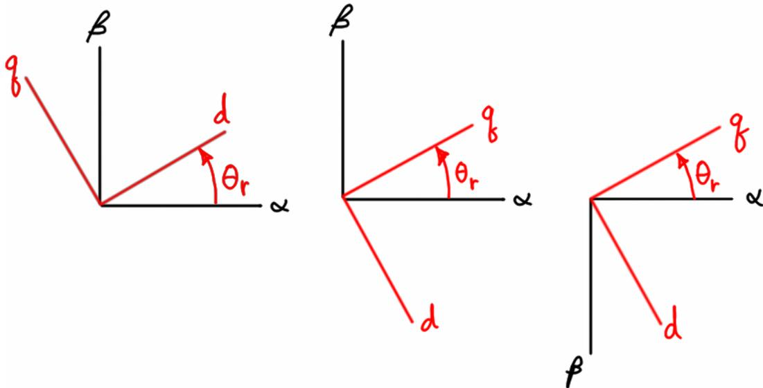
Figure E.1 – Some common axes and rotor angle conventions.
