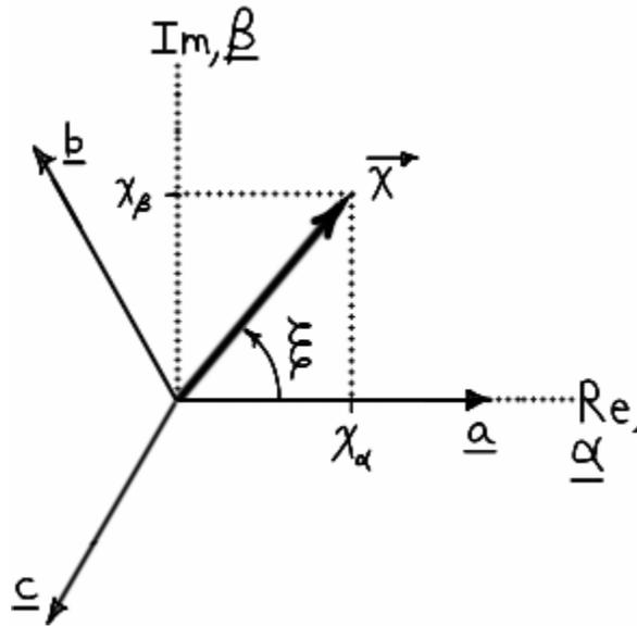
**Figure 3.33 – Space vector in stationary reference frame showing phase axes.**
