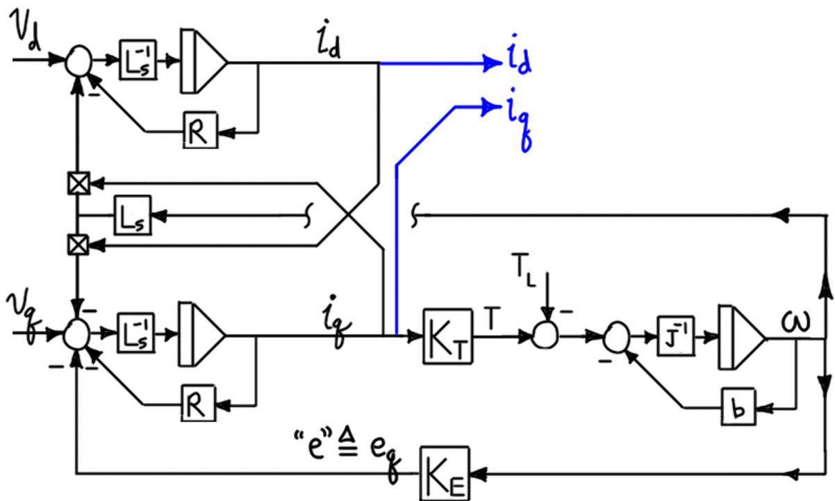
Figure 5.31 – Simulation diagram for BPMS motor in synchronous frame.
