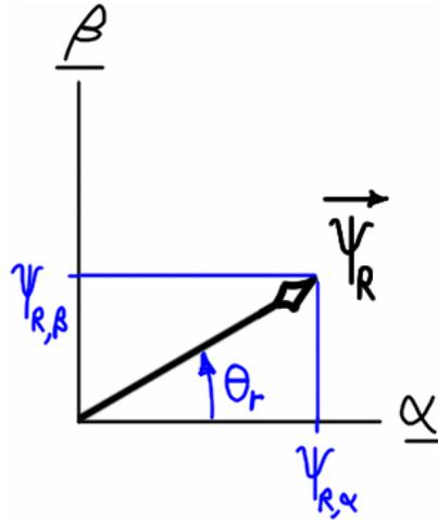
**Figure 6.2 – Rotor position estimation via rotor-stator flux linkage estimation.**
