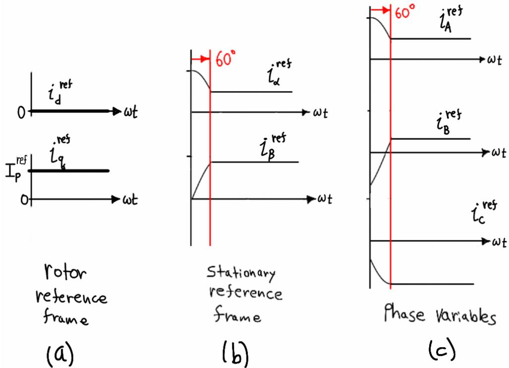
Figure 5.9 – Comparison of reference signals; rotor locked.
