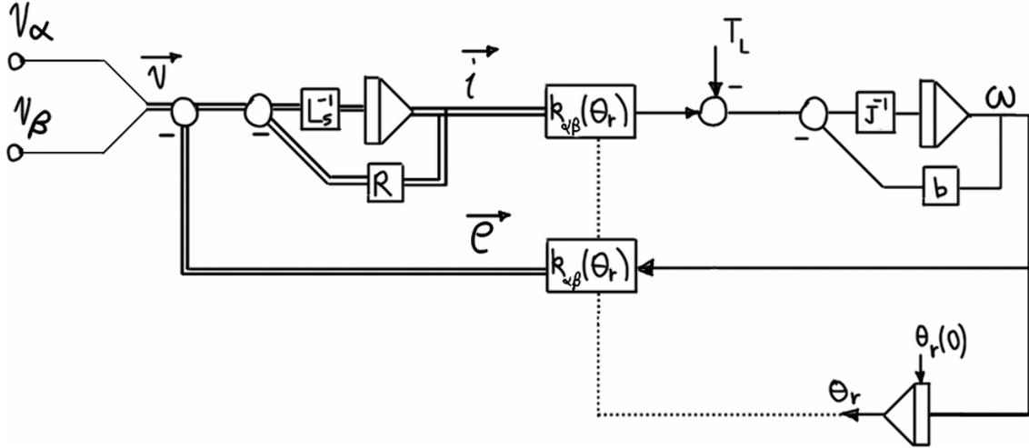
Figure 3.47 – Simulation diagram for BPMS motor in stationary frame (SV representation).
