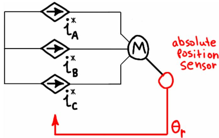
Figure 5.1 – Torque control of sinusoidal motor.
