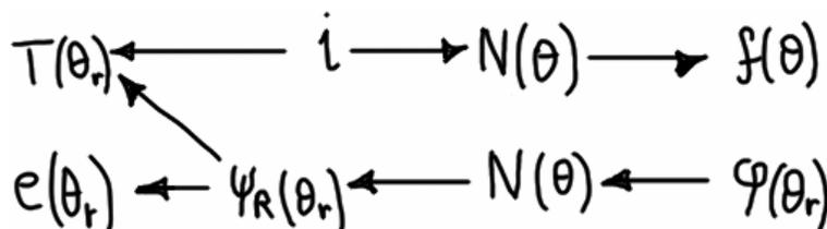
Figure C.21 – Torque and bEMF in terms of rotor-stator flux linkage.
