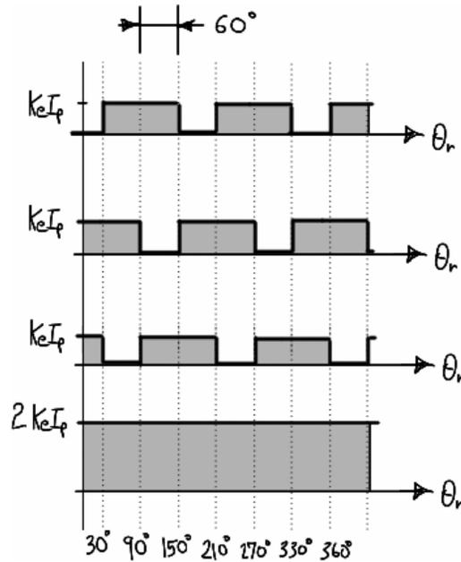
**Figure 2.32 – Torque production in trapezoidal BPMS motor.**
