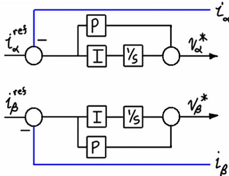
**Figure 5.26 – Stationary regulator in stationary frame.**
