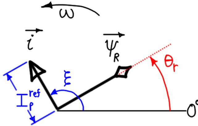
Figure 5.5 – SV diagram for most efficient torque production; stationary frame.
