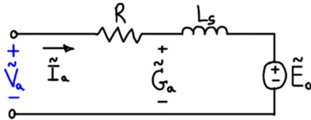
Figure 3.16 – Single-phase equivalent circuit.
