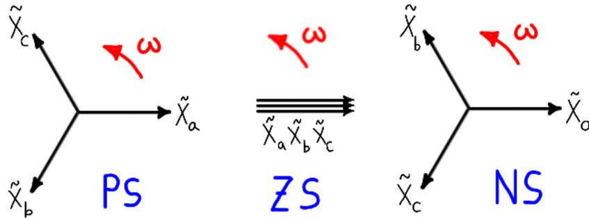
**Figure D.1 – Phasor diagrams for positive-, zero-, and negative- sequence sets.**
