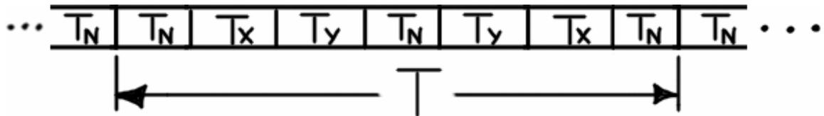
Figure 4.37 – One period on a second improved switching scheme.
