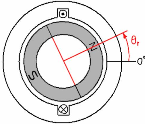
Figure C.14 – CFP winding with ideal squarewave rotor.
