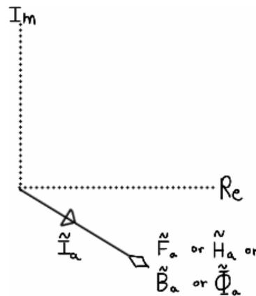
**Figure 3.20 – Time relationship between phase current and stator-produced magnetic quantities.**
