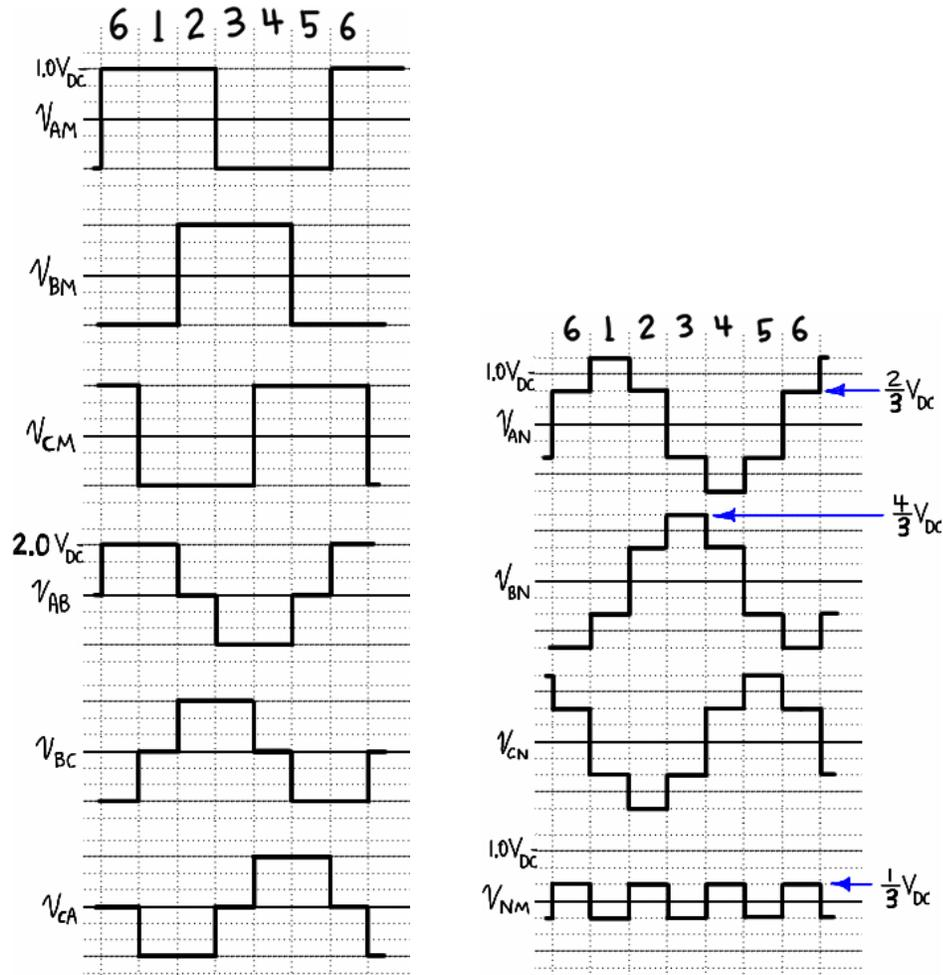
**Figure 4.23 – Voltage waveforms for  $180^\circ$  six-step squarewave inverter.**
