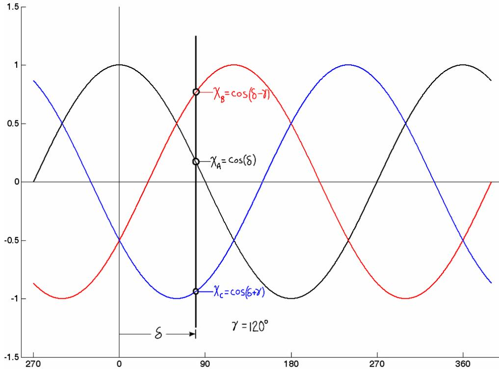
**Figure 3.6 – One electrical cycle of unit-amplitude, balanced sinusoidal general quantities.**
