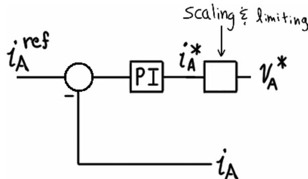
**Figure 4.15 – Ramp-comparison current regulator for one phase.**
