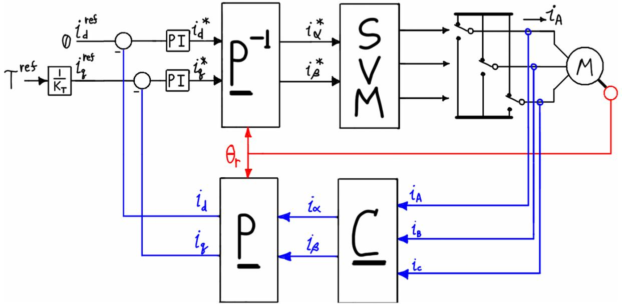
Figure 5.13 – Torque control of sinusoidal motor in rotor reference frame using SVM.
