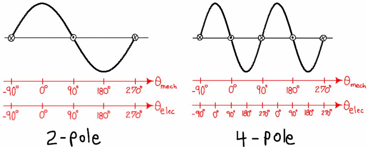
Figure 3.12 – Simplified developed view of a four pole motor.
