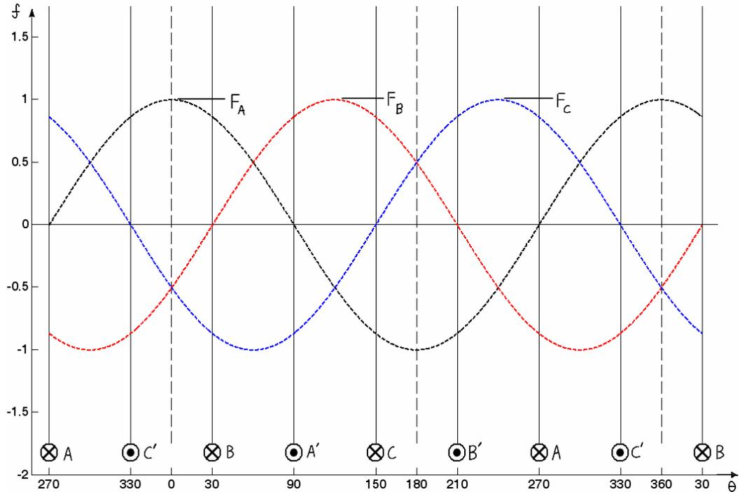
**Figure 3.4 – Developed view showing superimposed MMF distributions of all phases.**
