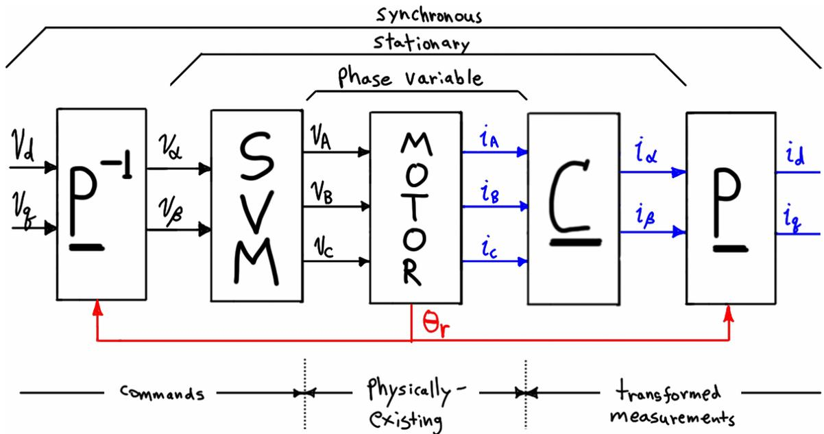
Figure 5.24 – Model of motor load (ideal inverter) viewed from three perspectives.
