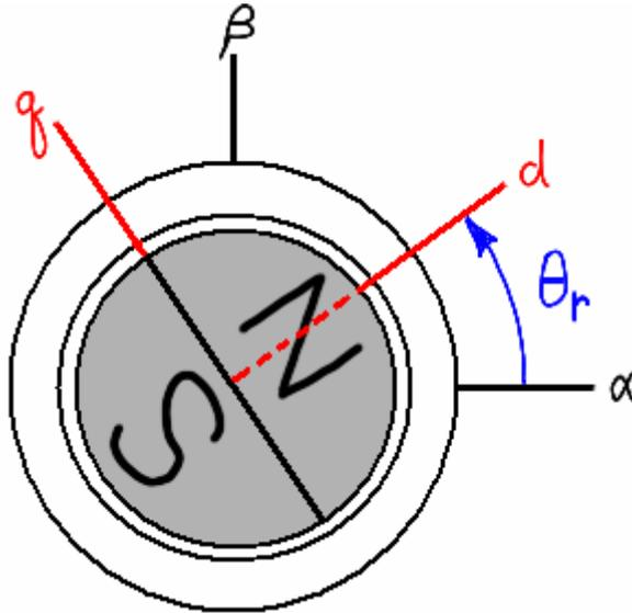
Figure 3.34 – Definition of rotor reference frame.
