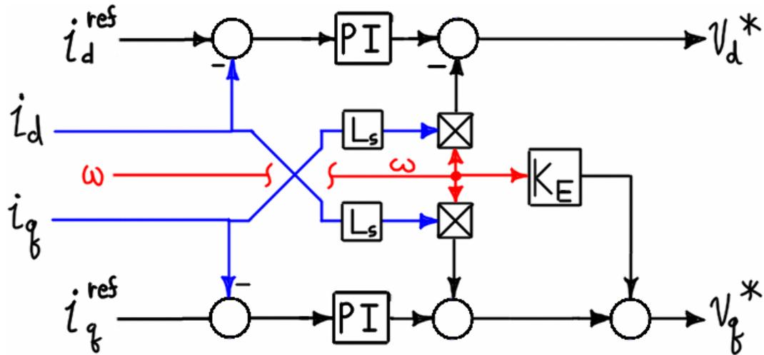
Figure 5.32 – bEMF offset and d-q current decoupling controller in synchronous frame.
