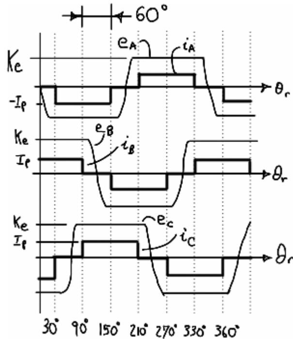
Figure 2.31 – Back-EMF and drive current for trapezoidal BPMS motor.
