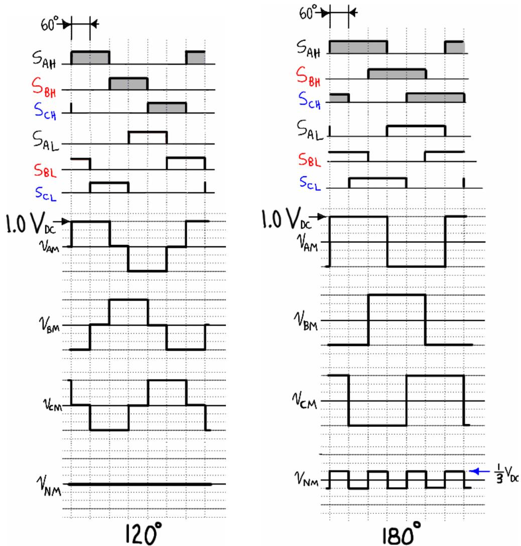
Figure 4.9 – Gating and POLE voltages for ideal 120° and 180° six-step inverters.
