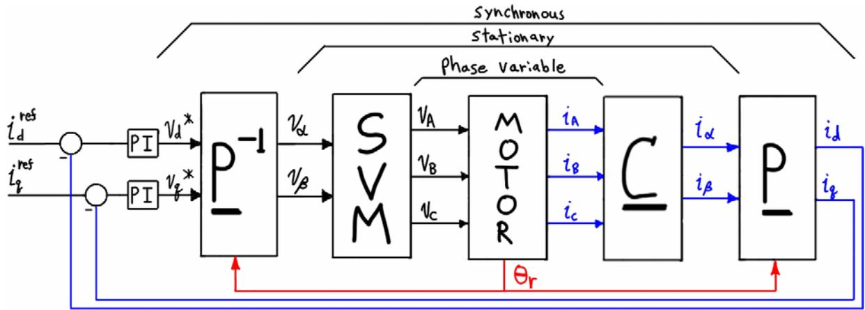
Figure 6.9 – FOC block diagram.
