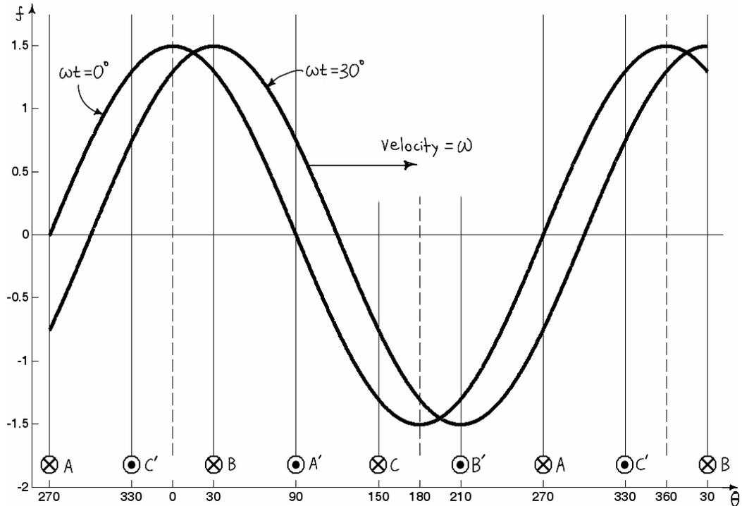
**Figure 3.9 – Developed view showing stator MMF waves of Figure 3.7 and Figure 3.8.**
