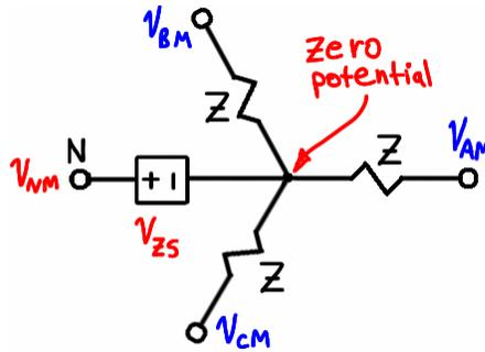
**Figure D.6 – Neutral voltage of load is common mode voltage of source.**
