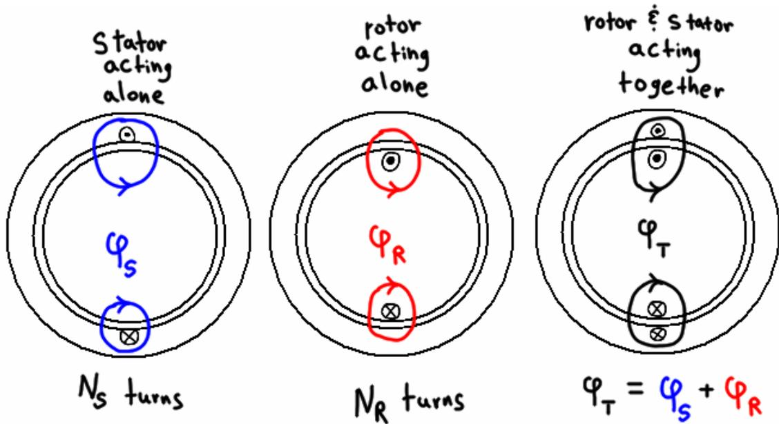
Figure A.1 – Stator, rotor, and total flux linkage.
