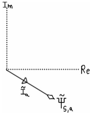
**Figure 3.21 – Time relationship between phase-A current and stator self flux linkage.**
