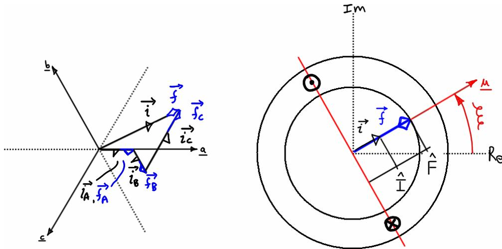
**Figure 3.27 – Equivalent MMF produced by coil with axis aligned with resultant MMF (c.f. Figure 3.24).**
