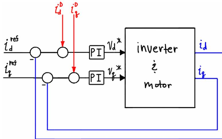
**Figure 5.33 – Top-level model of rotor-oriented FOC (with decoupling).**
