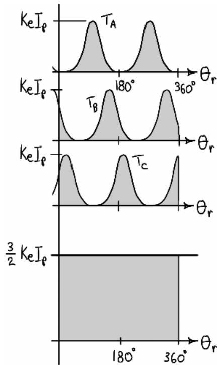
**Figure 2.30 – Torque production in sinusoidal BPMS motor.**
