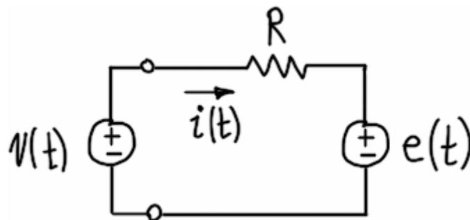
Figure 2.11 – Electrical model of coil connected to voltage source.
