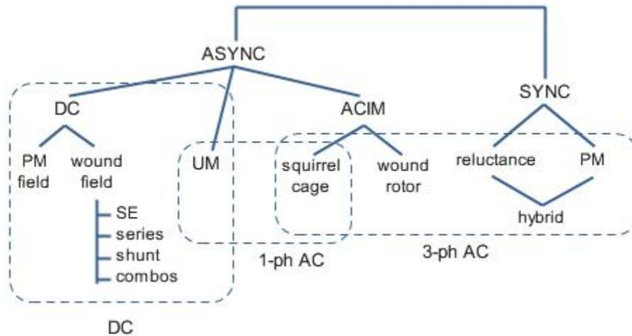
**Figure 2.5 – Motors categorized by power supply type.**
