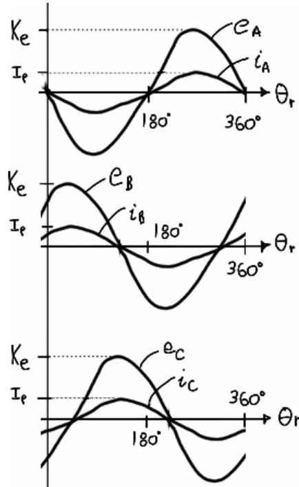
**Figure 2.29 – Back-EMF and drive current for sinusoidal BPMS motor.**
