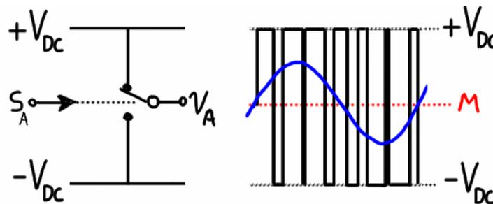
Figure 4.13 – Concept of PWM for one phase leg; not to scale.
