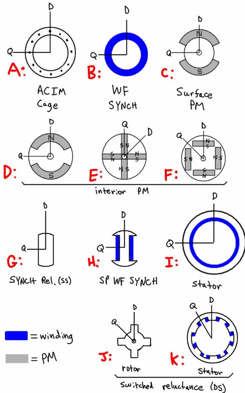
Figure 2.7 – Cross sections of some generalized synchronous motors.
