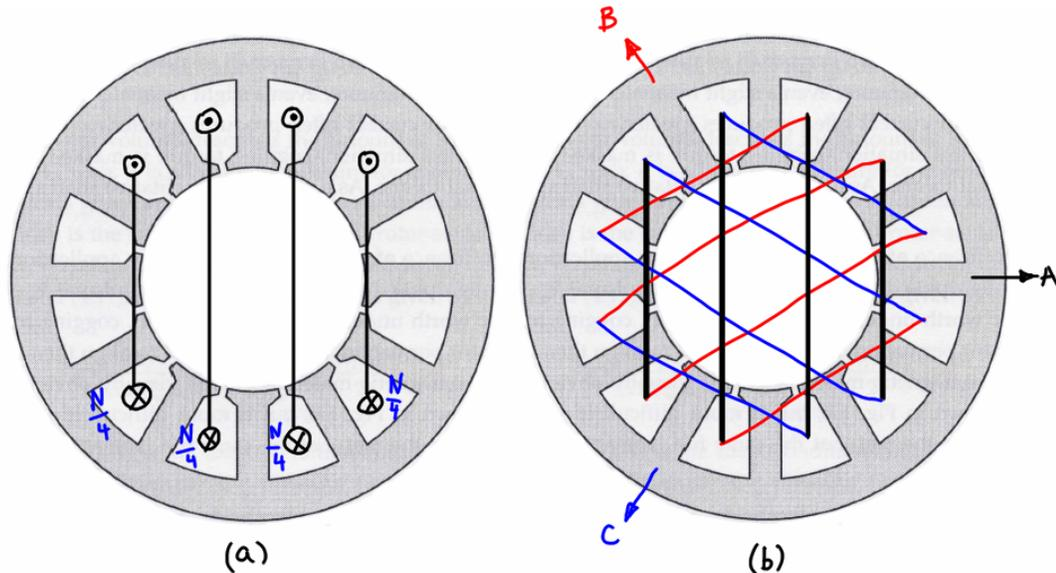
**Figure C.7 – Concentric winding of Figure C.6-b: (a) phase-A only; (b) all phases.**
