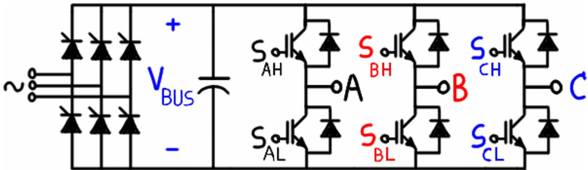
Figure 4.1 – VSI topology with controlled-rectifier front end.
