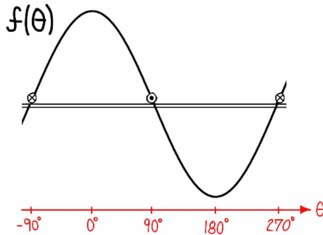
**Figure 3.3 – Developed view showing sinusoidal stator MMF distribution.**
