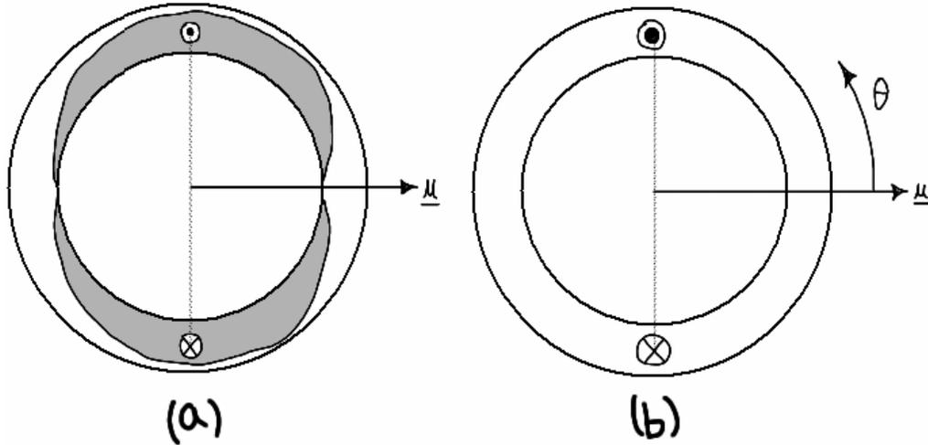
**Figure C.3 – Sinusoidal winding density.**
