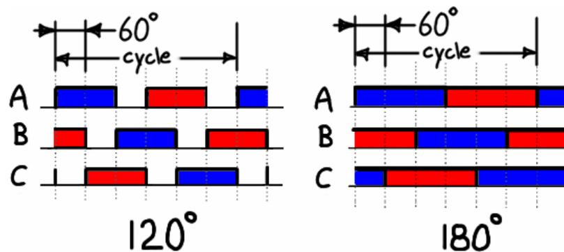
Figure 4.8 – Gating schemes for  $120^\circ$  and  $180^\circ$  inverters.
