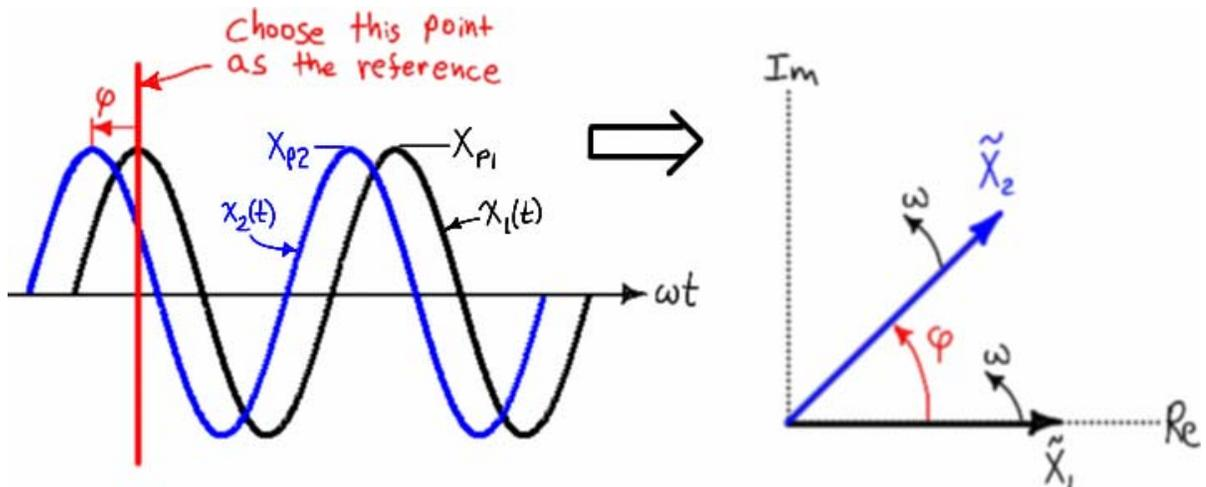
**Figure 3.39 – Time-domain waveform and corresponding phasor diagram.**
