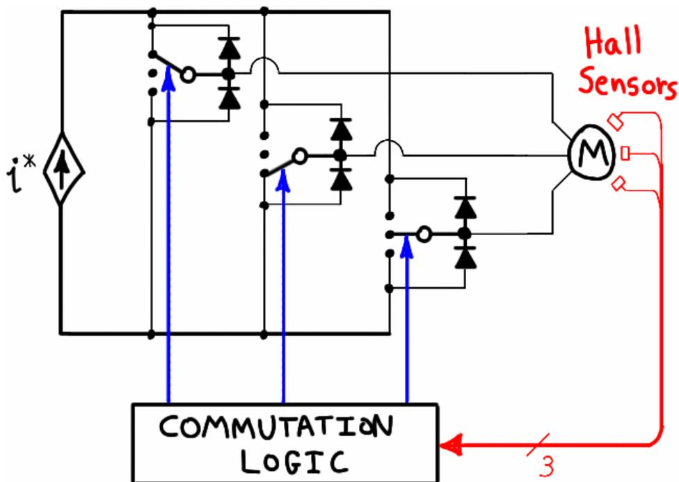
Figure 2.33 – Torque control of trapezoidal BPMS motor.
