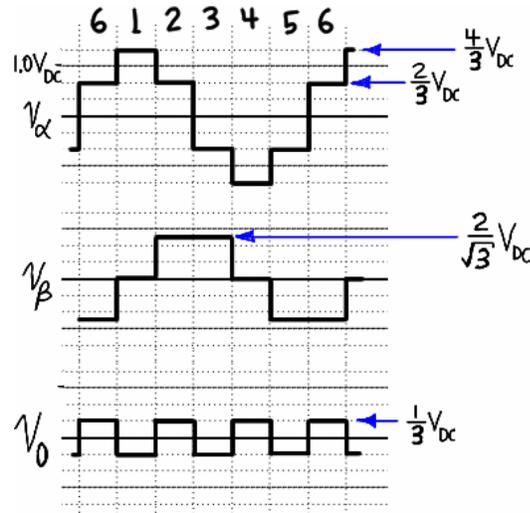
**Figure 4.27 – Transformed voltage waveforms for six-step 180° squarewave inverter.**
