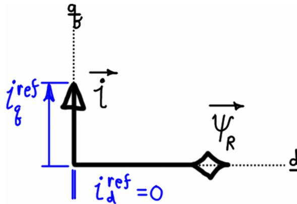
**Figure 5.7 – SV diagram for most efficient torque production; rotor frame.**
