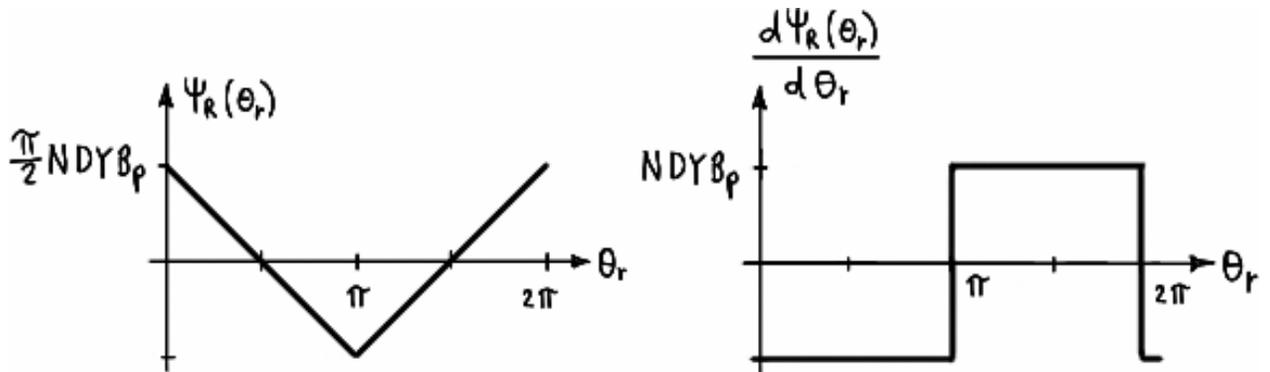
Figure C.15 – CFP winding with squarewave rotor: (a) rotor-stator flux linkage, and (b) its position-derivative.
