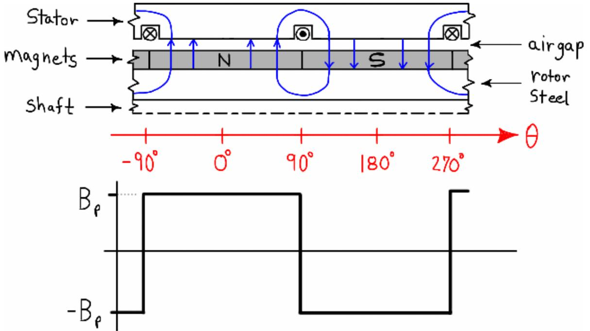
**Figure 2.13 – Developed view showing only ideal rotor flux density.**
