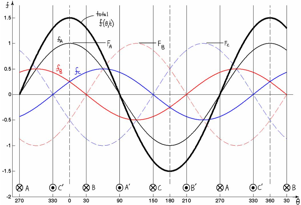
**Figure 3.7 – Developed view at zero electrical degrees.**
