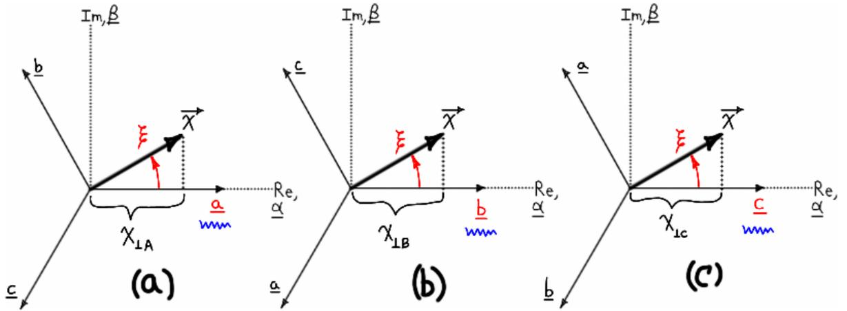
Figure 3.32 – Arbitrary SV referenced to axes of phases –A, -B, and –C.
