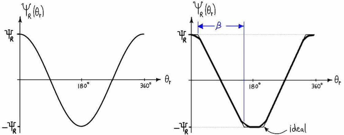
**Figure 2.26 – Rotor-stator flux linkage for a sinusoidal and arbitrary trapezoidal motor.**
