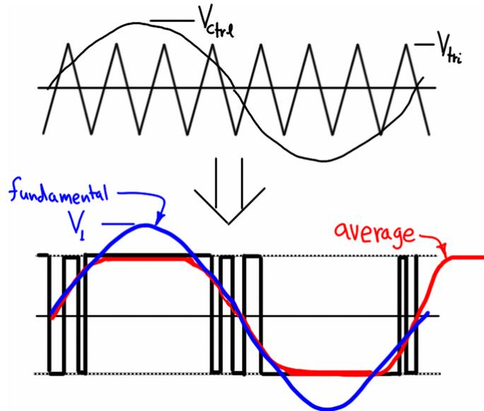
**Figure 4.17 – Overmodulation in carrier-based SPWM; not to scale.**
