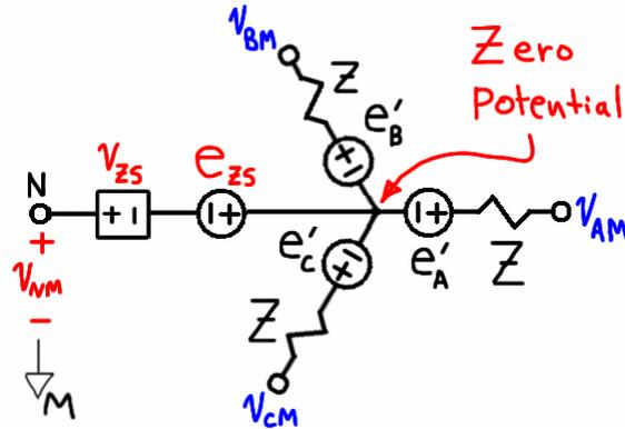
Figure D.9 – Load neutral voltage influence by ZS of source and bEMF.
