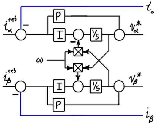
Figure 5.29 – Synchronous regulator in stationary frame.
