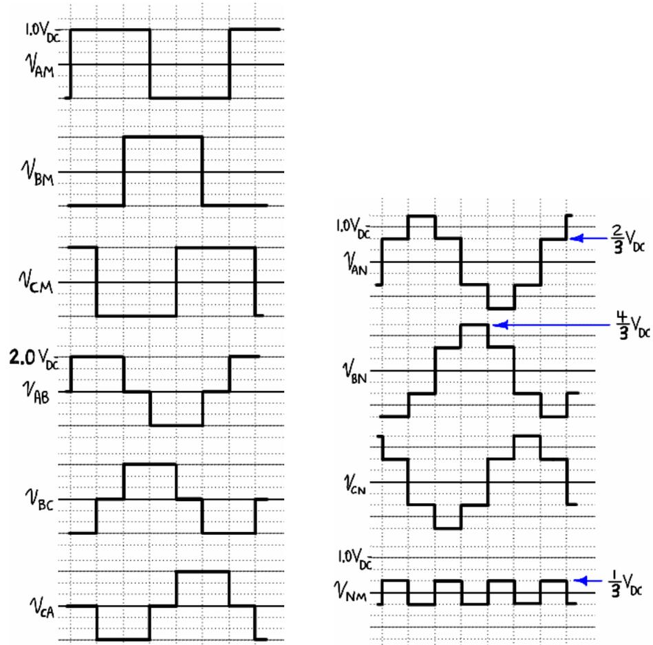
Figure 4.10 – Voltage waveforms for 180° six-step squarewave inverter.
