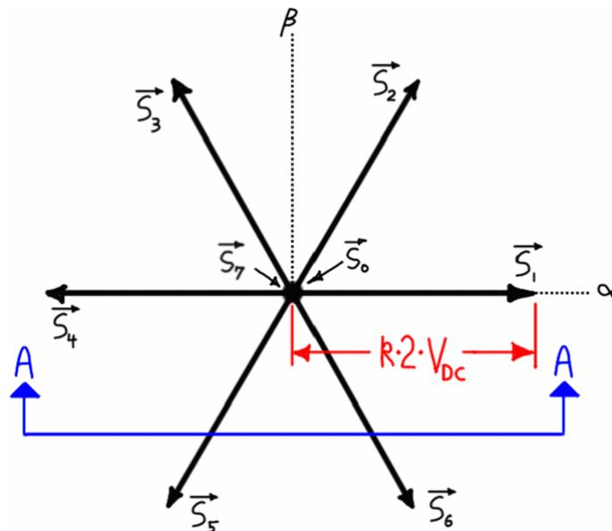
**Figure D.10 – Projection of base SVs of  $180^\circ$  inverter onto AB plane.**
