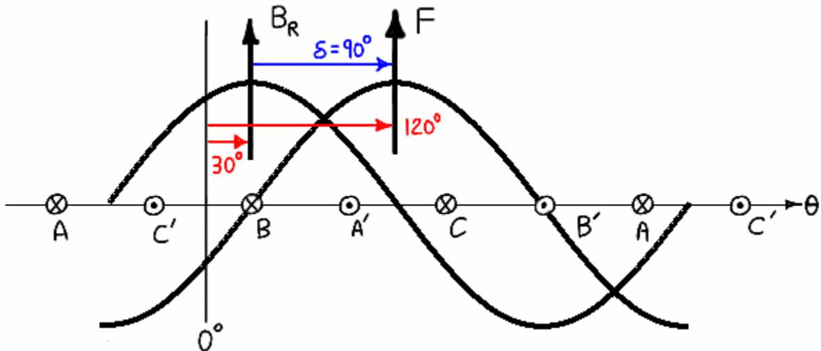
Figure 3.15 – Developed view showing rotor flux density and stator MMF.
