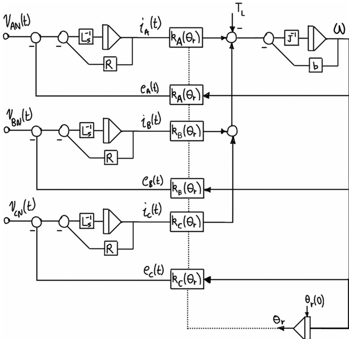
Figure 2.28 – Phase-variable simulation diagram of general motor.
