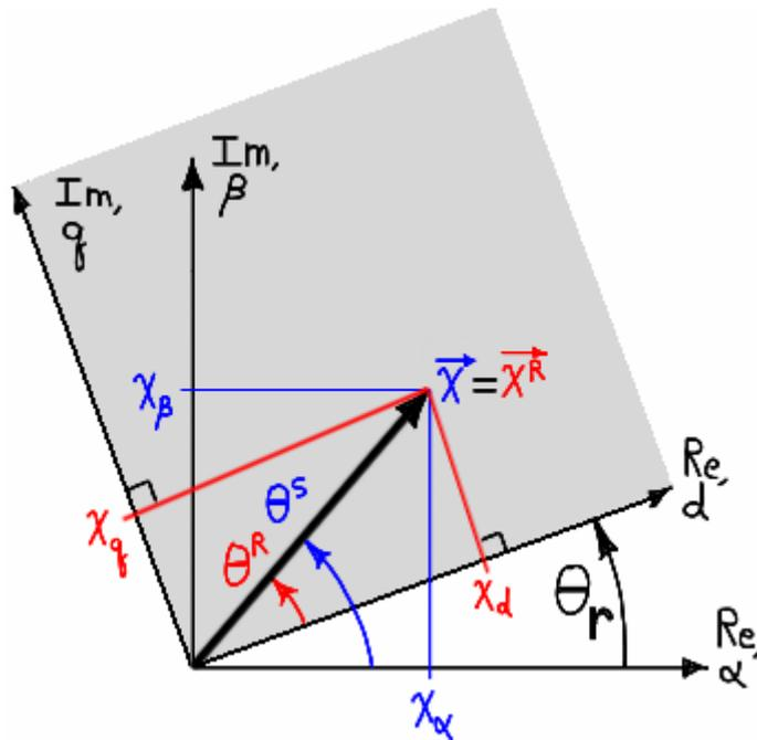
Figure 3.35 – SV in the stator and rotor reference frames.
