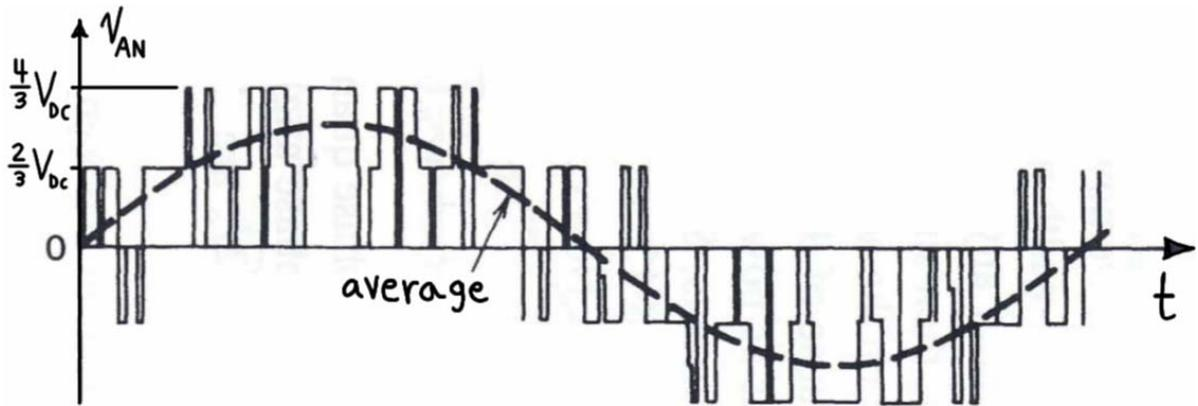
Figure 4.24 – Instantaneous phase-A line-neutral voltage in SPWM inverter.
