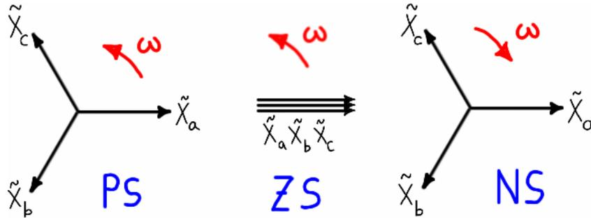
Figure D.2 – An alternate (but equivalent) interpretation of sequence sets.
