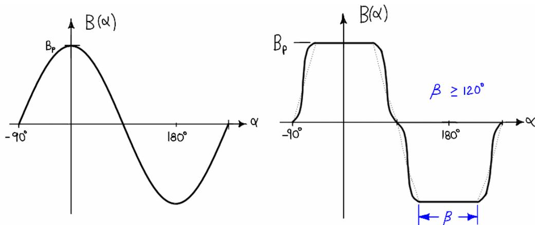
**Figure 2.21 – Airgap flux density profiles for two BPMS motors.**
