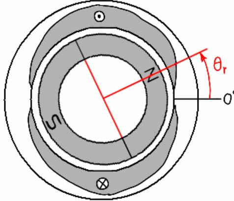
**Figure C.16 – Sinusoidal winding and squarewave rotor.**
