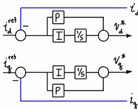
Figure 5.28 – Synchronous regulator in synchronous frame.
