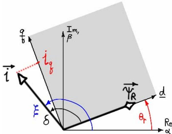
**Figure 3.45 – Torque production; stationary reference frame.**
