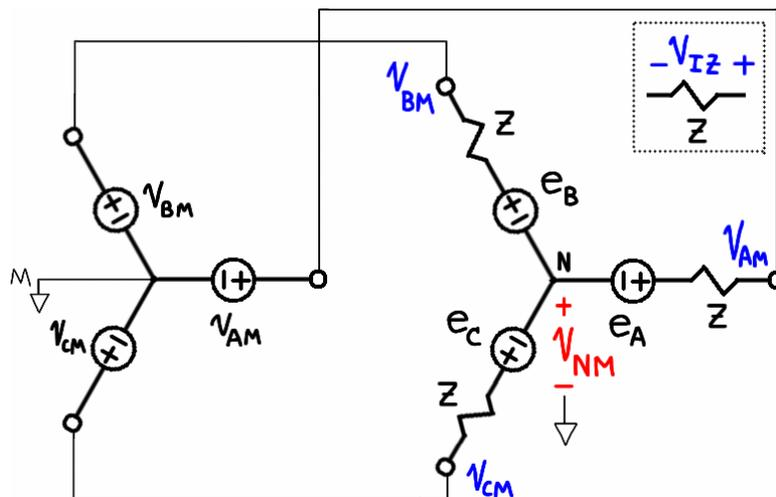
**Figure D.7 – Motor load driven by source.**
