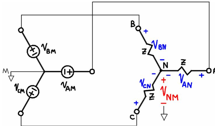
**Figure D.4 – Passive impedance load driven by source.**
