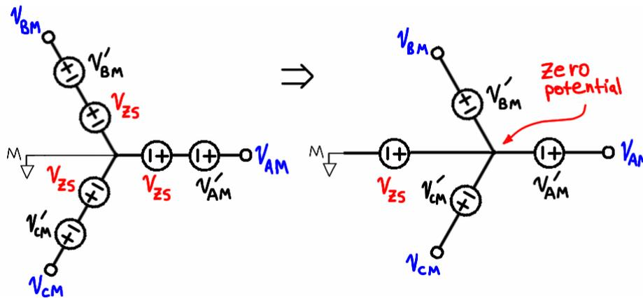
**Figure D.5 – Equivalent source showing that ZS is common-mode.**
