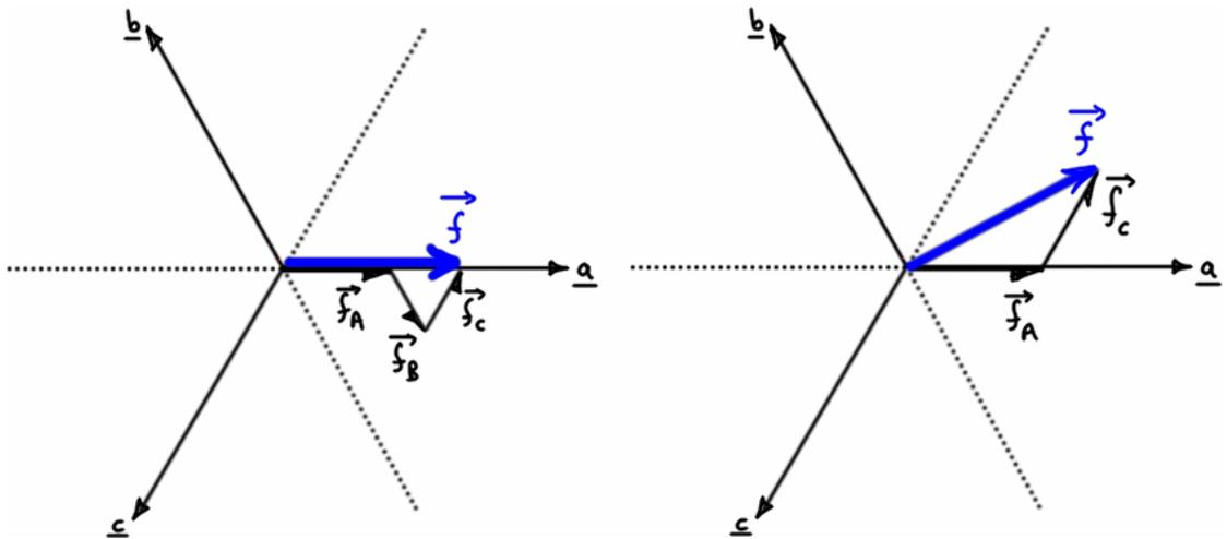
**Figure 3.26 – Addition of component MMF SVs to form total MMF SV (c.f. Figure 3.25).**
