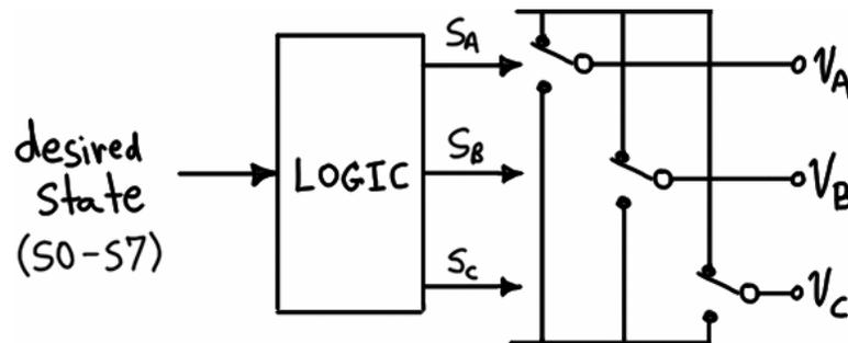
Figure 4.25 – Direct selection of inverter state.
