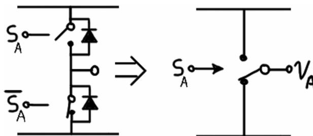
Figure 4.6 – Representation of leg in 180° inverter.
