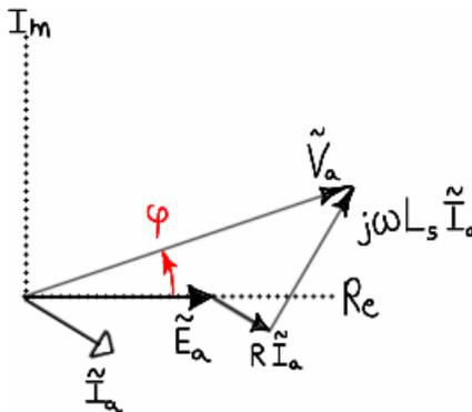
Figure 3.17 – Time phasor diagram of phase-A.
