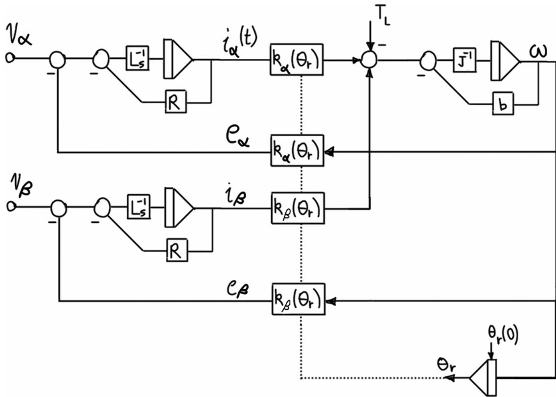
**Figure 3.46 – Simulation diagram for BPMS motor in stationary reference frame.**
