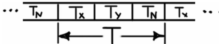
**Figure 4.35 – One period in a simple switching scheme.**
