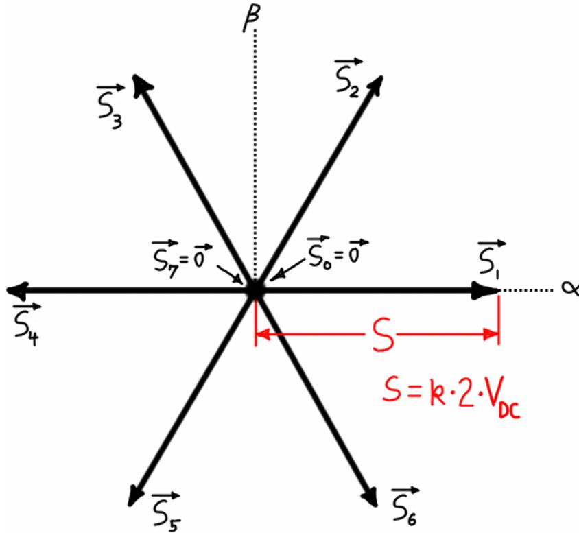
Figure 4.26 – Base SVs showing the states of a 180° inverter.
