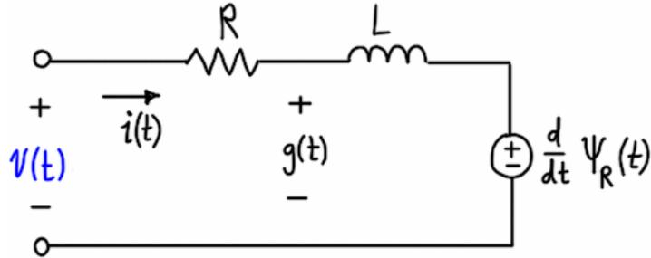
**Figure 2.17 – Per-phase electrical model of general brushless PM motor; explicit inductor.**
