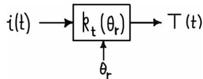
**Figure 2.23 – Simulation diagram for per-phase torque function.**
