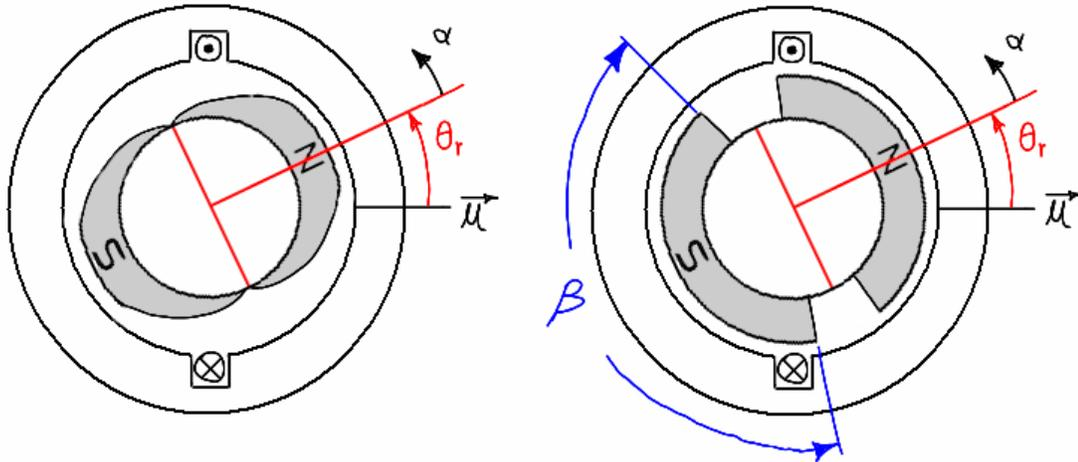
**Figure 2.20 – Elementary brushless PM motors with concentrated full-pitch winding.**
