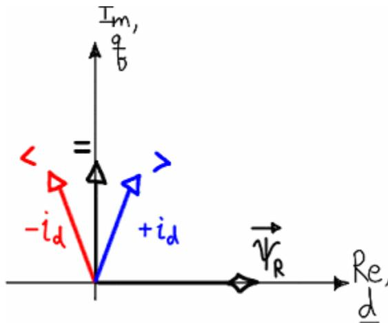
Figure 5.17 – Required position of stator current SV for maximum torque.
