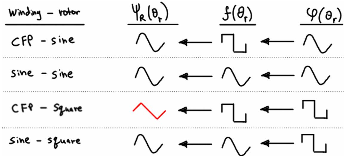
Figure C.18 – Summary of MMF and rotor-stator flux linkage results.
