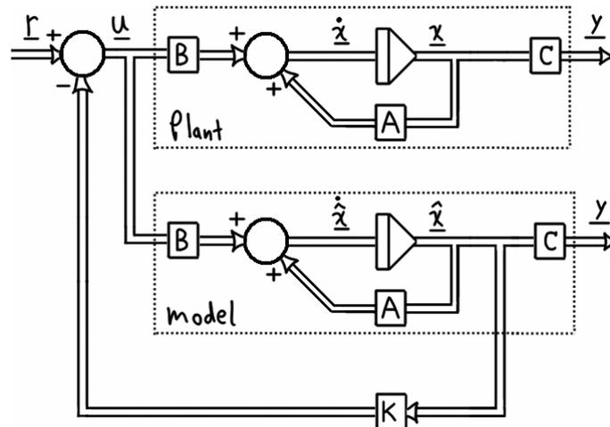
**Figure 6.6 – Full state feedback (open-loop estimator).**
