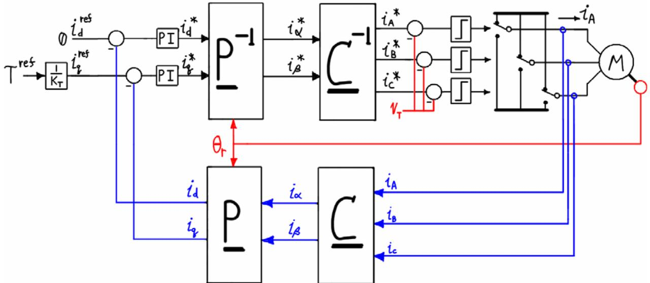
**Figure 5.12 – Torque control of sinusoidal motor; rotor reference frame.**
