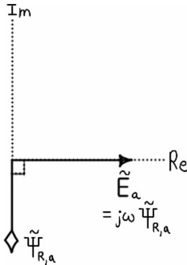
**Figure 3.19 – Time relationship between flux linkage due to rotor and bEMF.**
