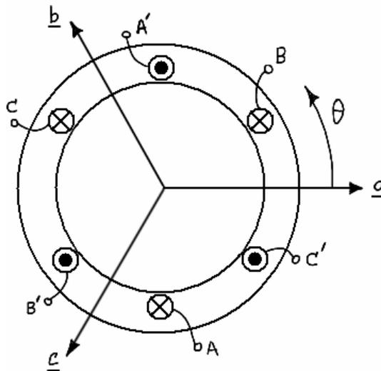
**Figure 3.1 – Stator of three-phase sinusoidal synchronous machine.**
