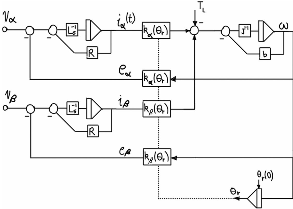
**Figure 6.8 – BPMS motor model in stationary frame.**
