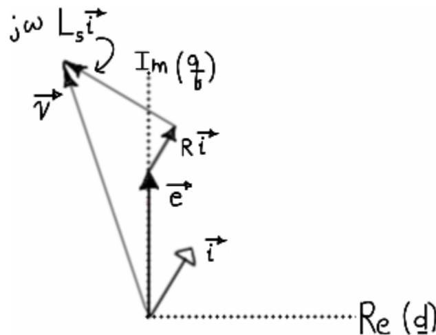
**Figure 3.49 – Steady-state SV diagram in rotor frame.**
