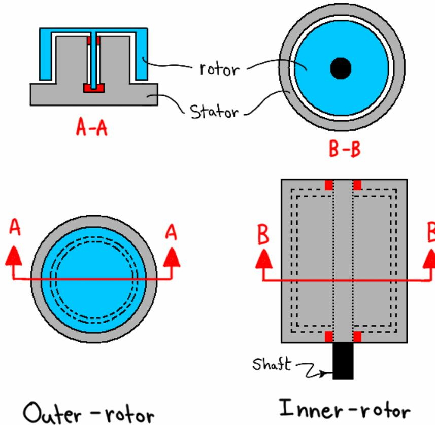
Figure 2.2 – Outer- and inner- rotor radial flux motors.
