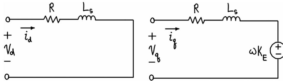
**Figure 5.34 – Compensated or approximate model of BPMS motor in synchronous frame.**
