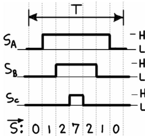
Figure 4.38 – Leg control signals; commanded SV in sextant  $s_{12}$ .
