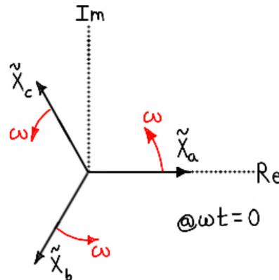
Figure 3.18 – Positive sequence phasor orientation.
