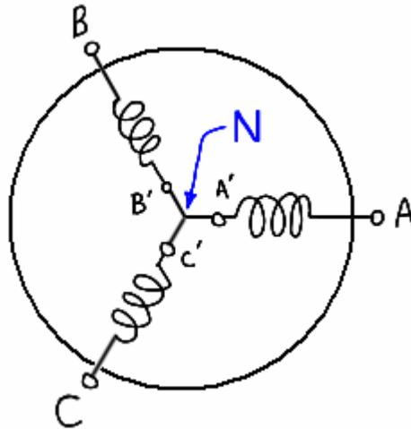
**Figure 3.2 – Three phase wye-connected stator with three phase terminals.**
