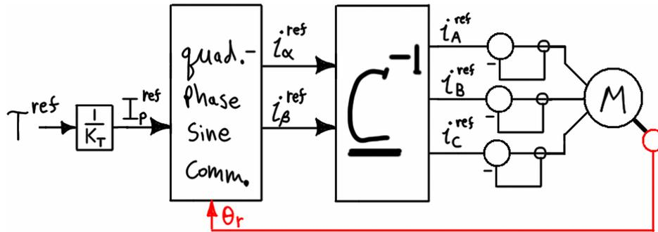
Figure 5.4 – Torque control in stationary reference frame.
