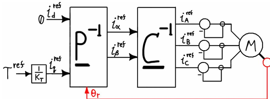
Figure 5.6 – Torque control in rotor reference frame.
