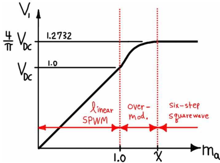
**Figure 4.18 – Fundamental gain and operating modes of carrier-based SPWM.**
