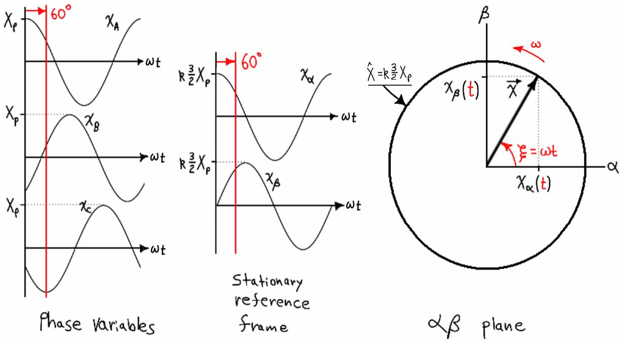
Figure 3.30 – Waveforms and SV trajectory for balanced sinusoidal phase variables.
