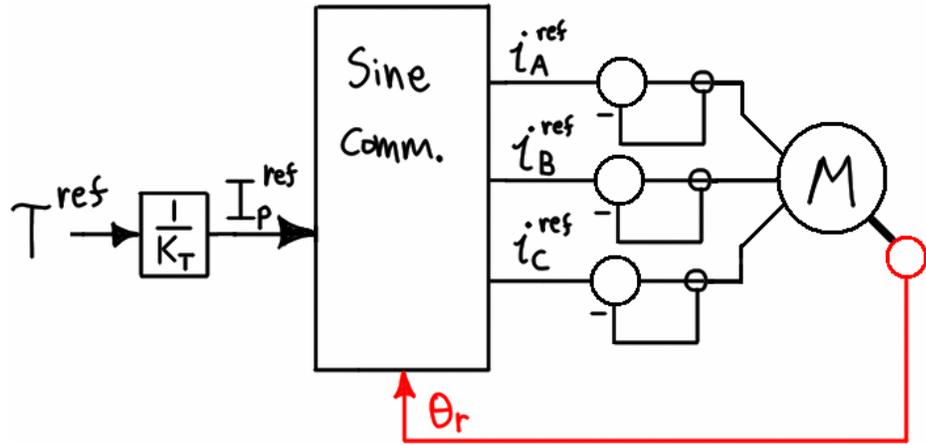
Figure 5.3 – Torque control of sinusoidal motor; phase variable form.
