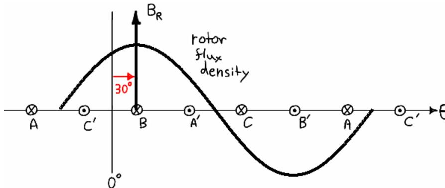
**Figure 3.13 – Developed view of two pole motor showing rotor flux density.**
