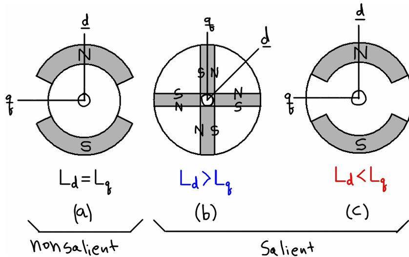
**Figure 5.15 – Rotor types: (a) nonsalient (surface magnet); (b), (c) salient (interior magnet).**
