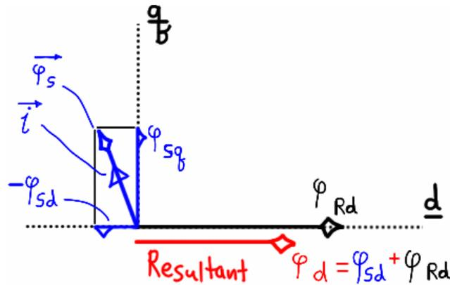
Figure 5.21 – Flux weakening in the rotor reference frame.
