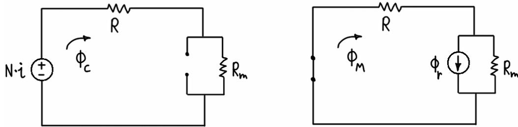
Figure 2.16 – Components of total flux (cf. Figure 2.15).
