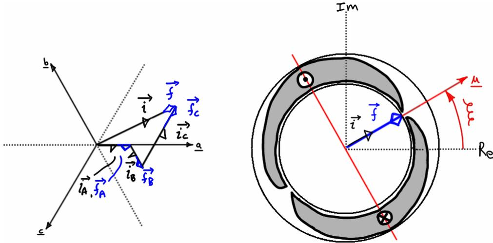
**Figure 3.28 – Axis of rotating amp-turn distribution cophasal with current and MMF SVs.**
