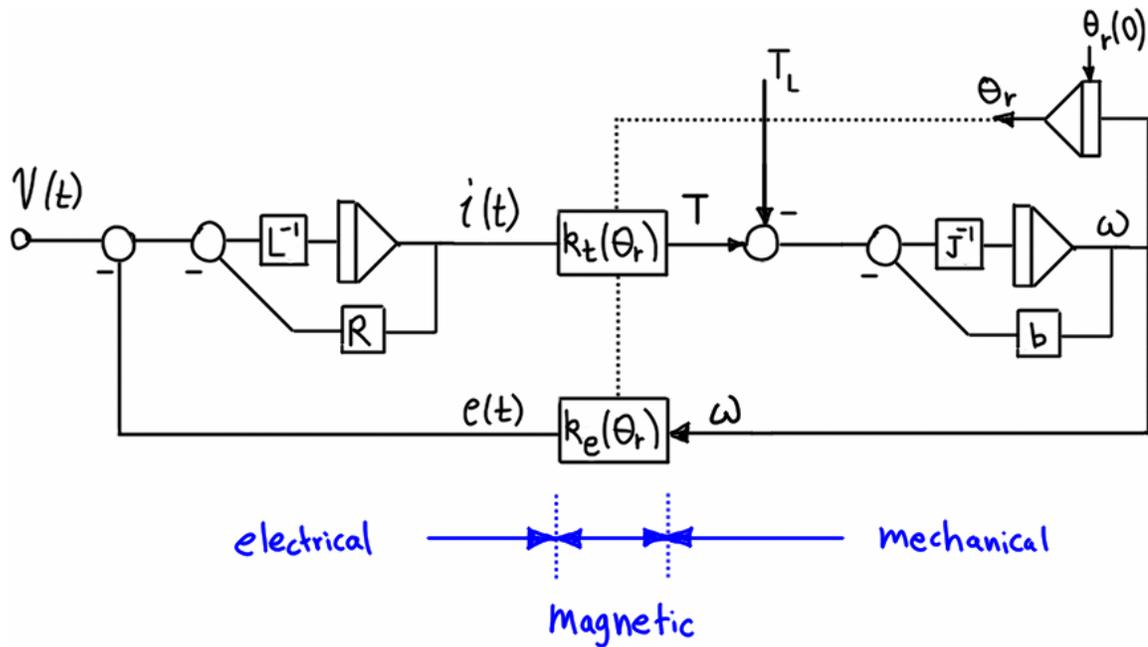
**Figure 2.27 – Simulation diagram of general motor.**
