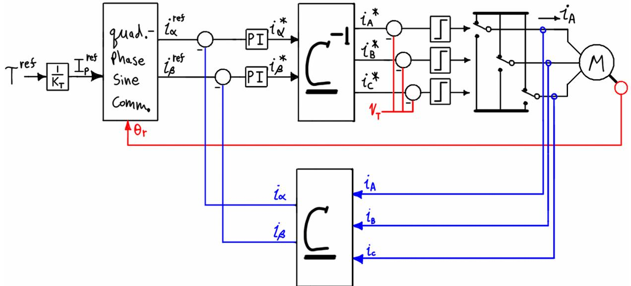
**Figure 5.11 – Torque control of sinusoidal motor; stationary reference frame.**
