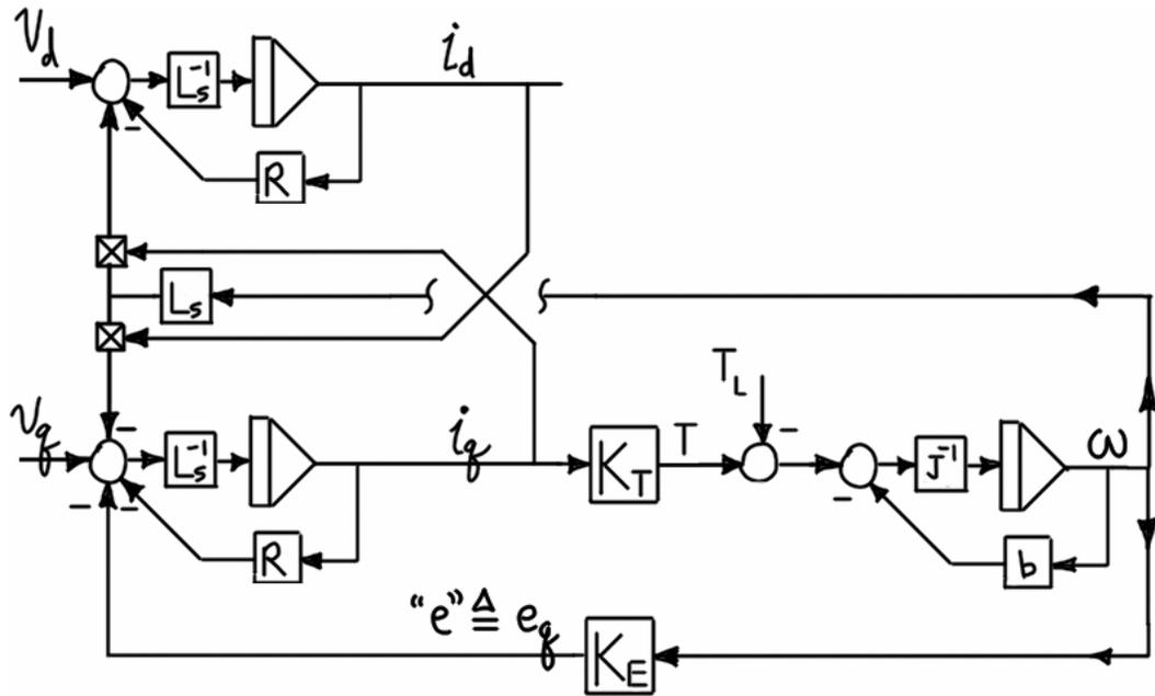
Figure 3.48 – Simulation diagram for BPMS motor in synchronous reference frame attached to rotor.
