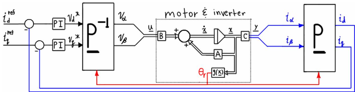
Figure 6.10 – State-space model of motor and inverter.
