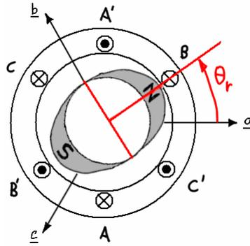
Figure 3.14 – Cross section of two pole motor.
