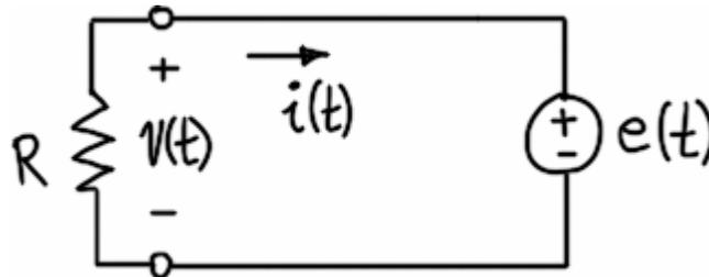
**Figure 2.9 – Electrical model of ideal coil shunted by an external resistance.**
