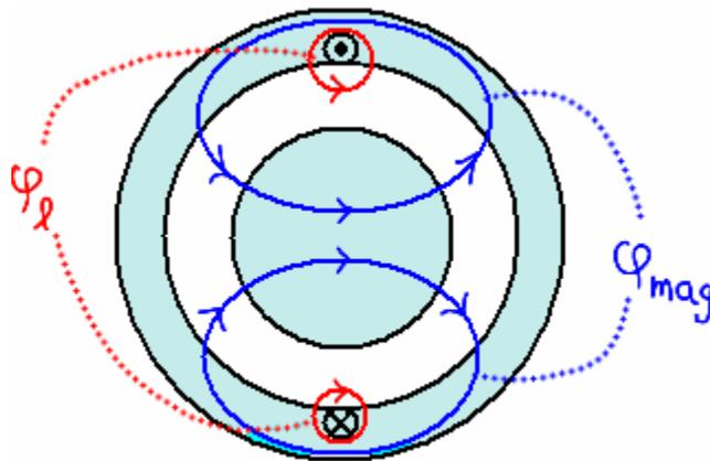
**Figure B.1 – Magnetizing and leakage paths of stator flux.**
