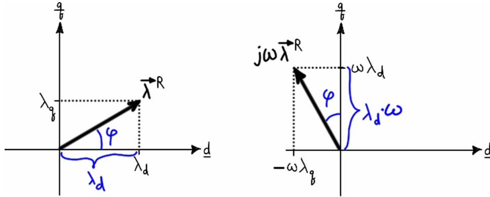
Figure 3.42 – Coupling between d- and q- axes in voltage equations.
