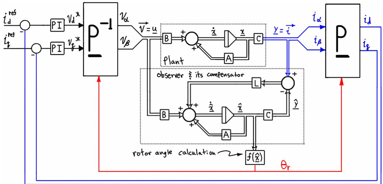
Figure 6.11 – Sensorless FOC using observer.
