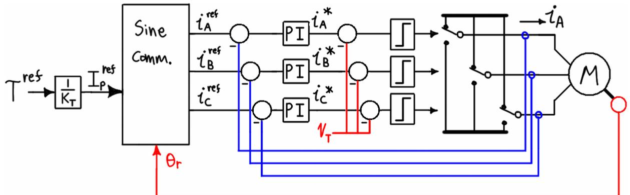
**Figure 5.10 – Torque control of sinusoidal motor; phase-variable form.**
