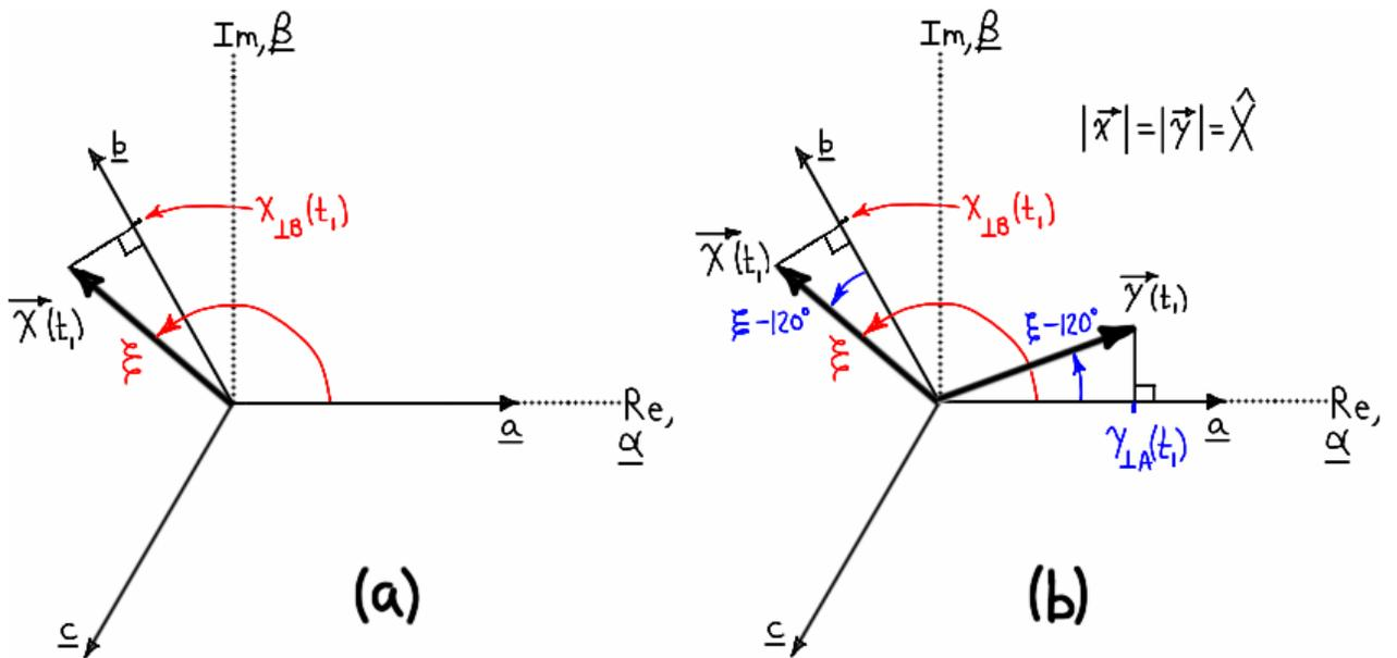
**Figure 3.31 – SV projection onto phase axes: (a) actual; (b) alternative.**
