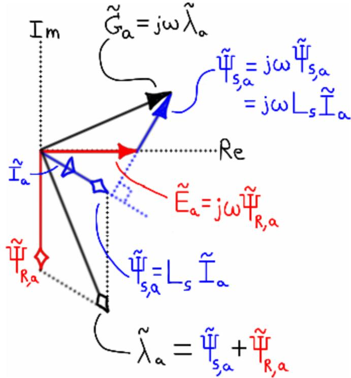
**Figure 3.23 – Time relationships between flux linkages and induced voltages; lagging PF.**
