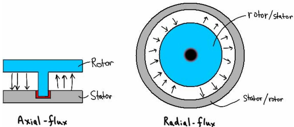
**Figure 2.1 – Radial- and axial- flux motors.**
