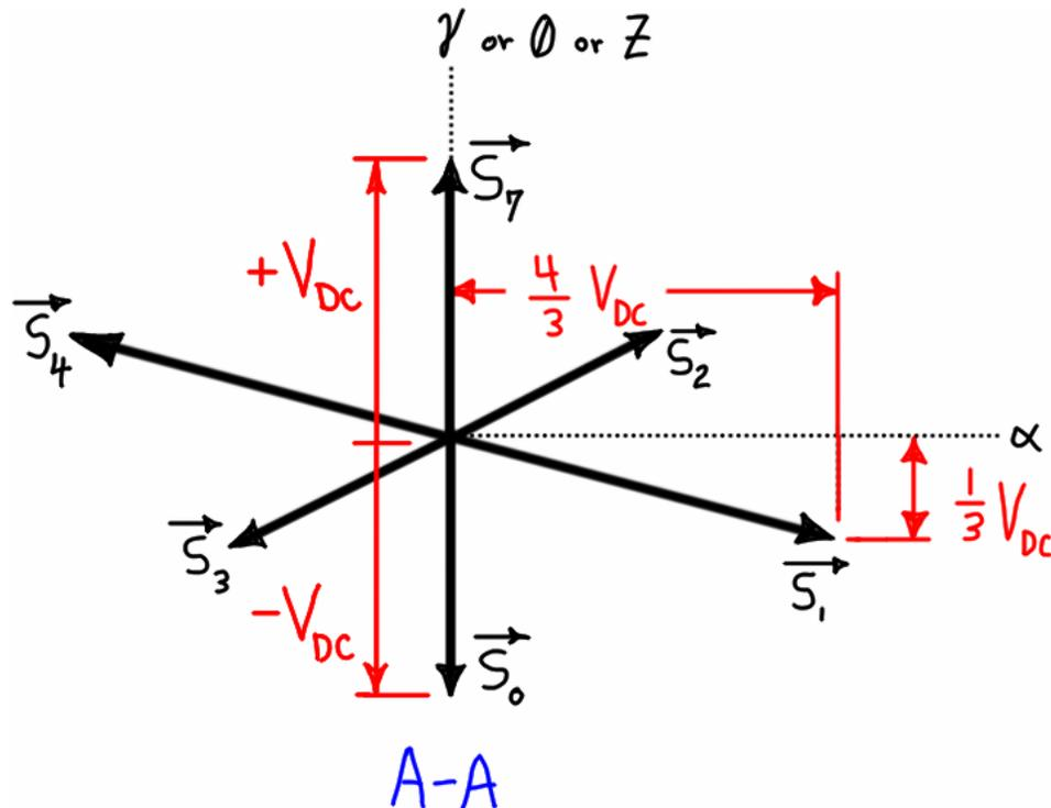
Figure D.11 – 3-D base vectors of 180° inverter.
