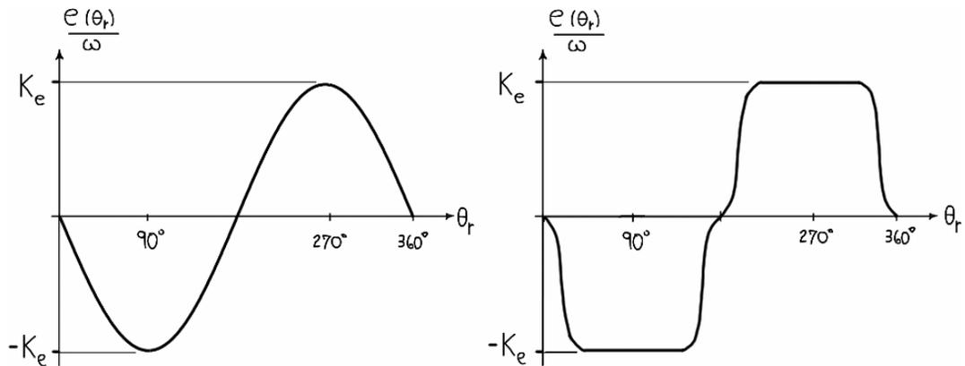
**Figure 2.24 – Back EMF functions of a sinusoidal and arbitrary trapezoidal motor.**
