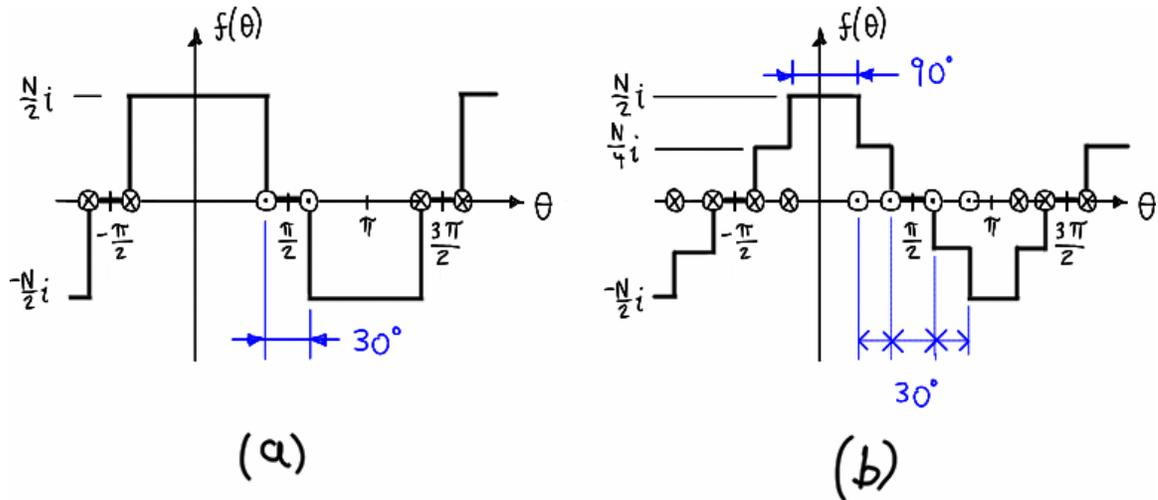
Figure C.10 – MMF of (a) distributed full-pitch winding; (b) distributed short-pitched winding.
