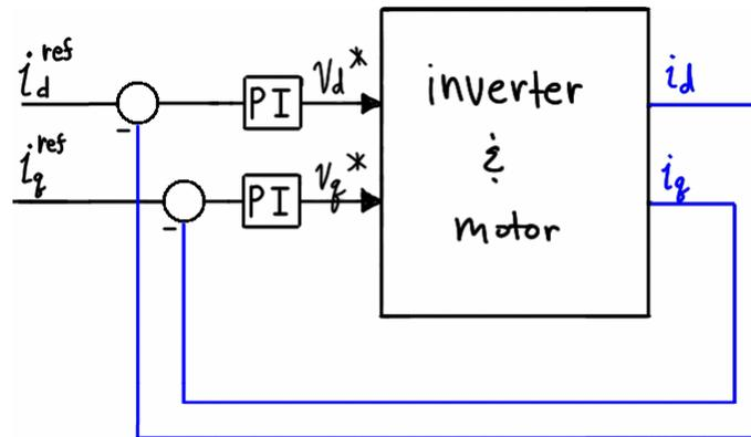
Figure 5.30 – Top-level model of rotor-oriented FOC.
