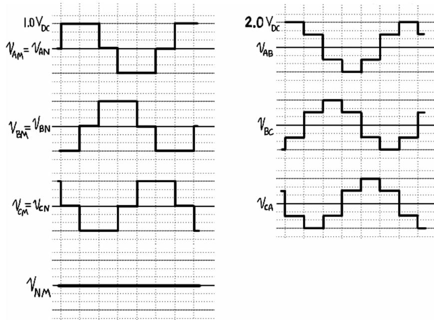
Figure 4.11 – Ideal voltage waveforms for 120° six-step squarewave inverter with resistive load.
