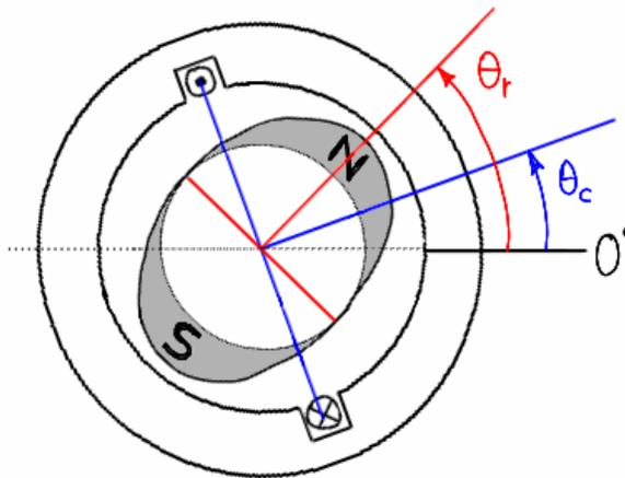
**Figure C.12 – Full-pitch coil axis at  $\theta_c$  and sinusoidal rotor at position  $\theta_r$ .**
