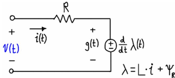
**Figure 2.19 – Per-phase electrical model of general brushless PM motor; implicit inductor.**
