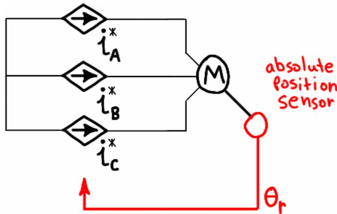
Figure 2.34 – Torque control of sinusoidal BPMS motor.
