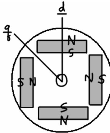
Figure 5.19 – Buried permanent magnet rotor.
