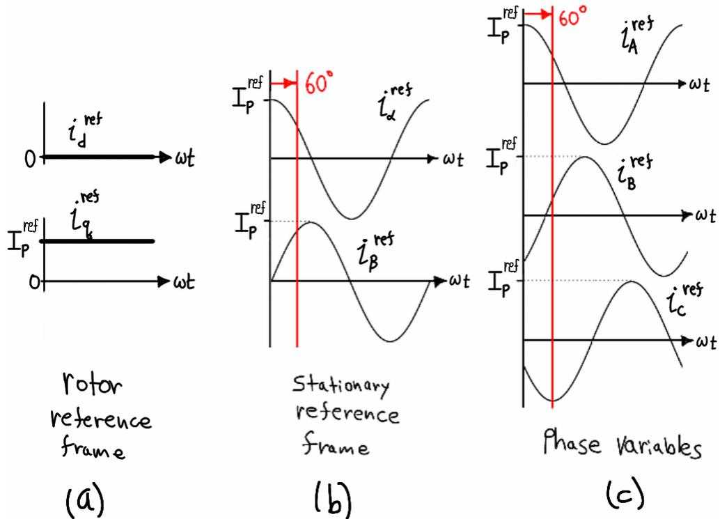
**Figure 5.8 – Comparison of reference signals under steady state operation.**
