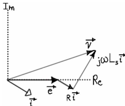
**Figure 3.41 – SV diagram of synchronous motor in stationary frame (steady state).**
