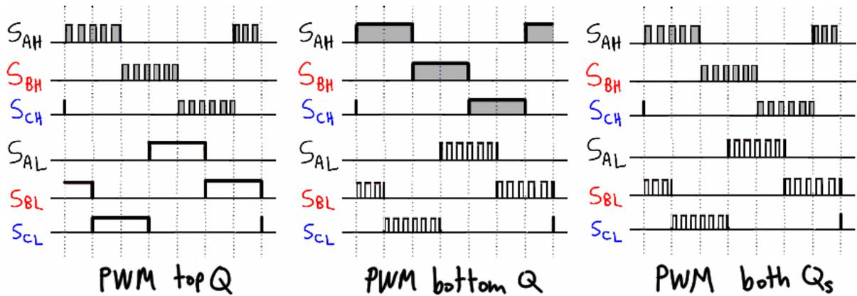
Figure 4.12 – Commutation and PWM configurations in 120° inverter.
