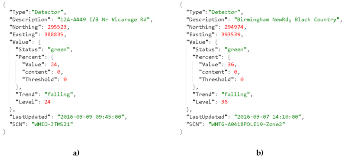
Figure 4.1 – Birmingham City Council sensor data source examples. a) flow sensor reading; b) average speed sensor reading
