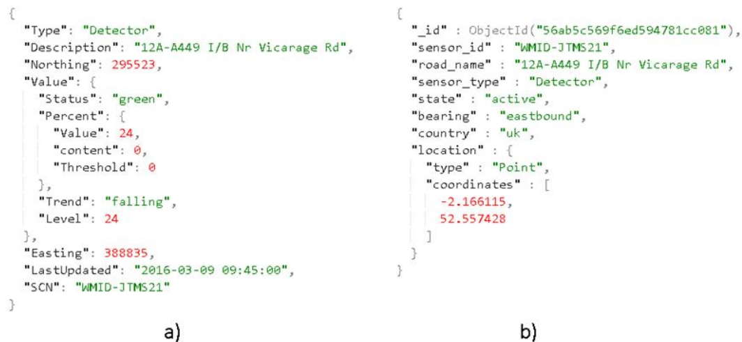
Figure 5.5 – Traffic sensor metadata harmonization example from raw data (a) to harmonized data (b)
