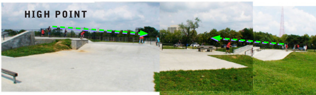
FIGURE 5.41: Creating a high point for a street course helps all skaters see each
