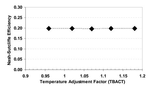
Figure 5.6. Temperature Adjustment Factor (TBACT) model efficiency response for daily fecal bacteria prediction for Rock Creek
