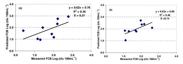
Figure 4.7. Measured fecal coliform bacteria (FCB) concentration model response for (a) Rock Creek, and (b) Deer Creek watersheds
