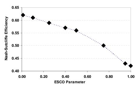
Figure 5.3. Soil evaporation compensation factor (esco) model efficiency response for daily flow for Richland gaging station
