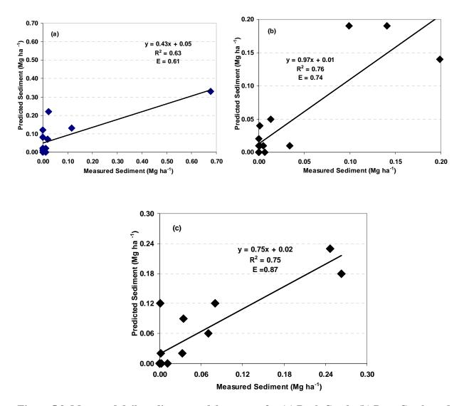
Figure 5.9. Measured daily sediment model response for (a) Rock Creek, (b) Deer Creek, and (c) Auburn watersheds
