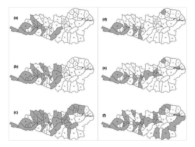
Figure 6.5. Distribution of watershed sub-basins for sediment BMP selection: target method (a) 10%, (b) 25%, (c) 50% and random method (d) 10%, (e) 25%, and (f) 50%
