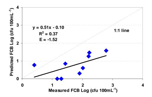
Figure 3.4. Measured fecal coliform bacteria (FCB) concentration model response
