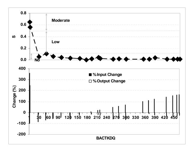
Figure 3.5. LHS method: bacteria partition coefficient in surface runoff (BACTKDQ) relative sensitivity index (S) response
