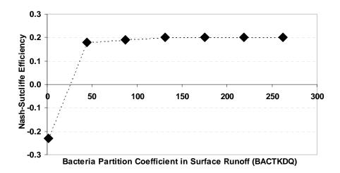
Figure 5.5. Bacteria Partition Coefficient in Surface Runoff (BACTKDQ) model efficiency response for daily fecal bacteria prediction for Rock Creek
