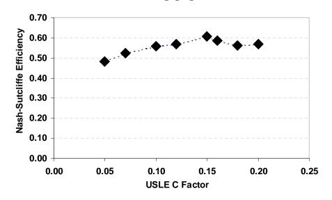
Figure 5.4. Universal soil loss equation (USLE) model efficiency response for daily sediment yield for Rock Creek
