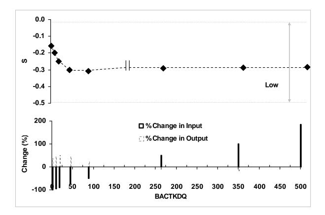
Figure 2.7. Bacteria partition coefficient in surface runoff (BACTKDQ) relative sensitivity index (S) response
