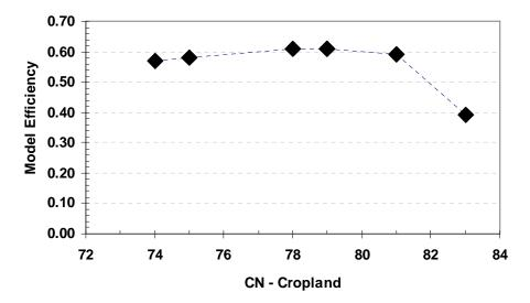
Figure 5.2. Cropland curve number (CN) and model efficiency response for daily flow for Richland gaging station.
