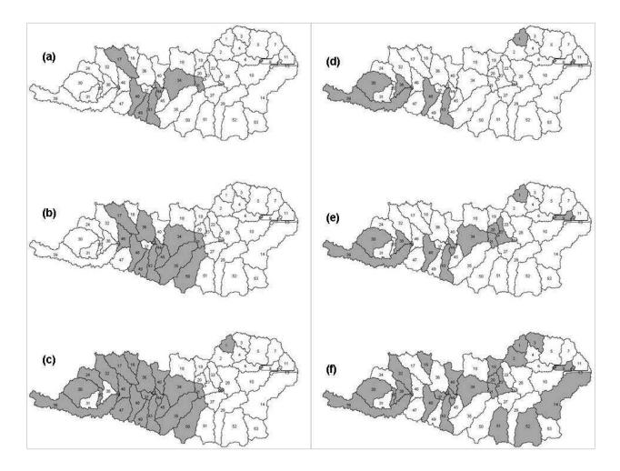
Figure 6.4. Distribution of watershed sub-basins for fecal bacteria BMP selection: target method (a) 10%, (b) 25%, (c) 50% and random method (d) 10%, (e) 25%, and (f) 50%
