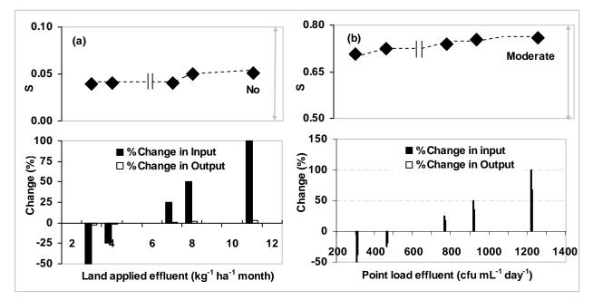
Figure 2.10. Septic source load application methods relative sensitivity response for (a) landapplied and (b) point load
