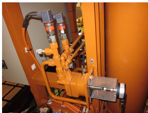
Figure 9. Hydraulic motor, input and output pressure transducers and the encoder coupled to the shaft.
