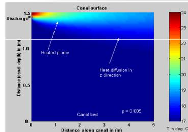
Model applied on Matlab shows temperature distribution profile through the depth
