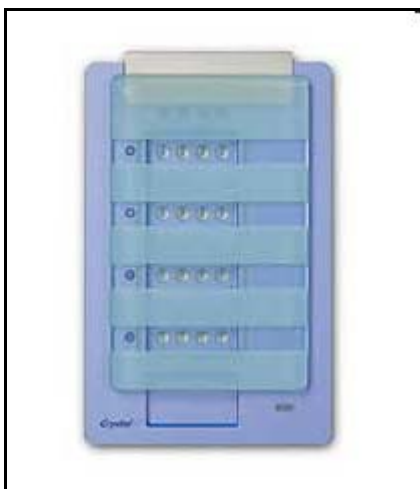
Figure 29: Crystal16 TM equipment (16 multiple-reactor system). 111
