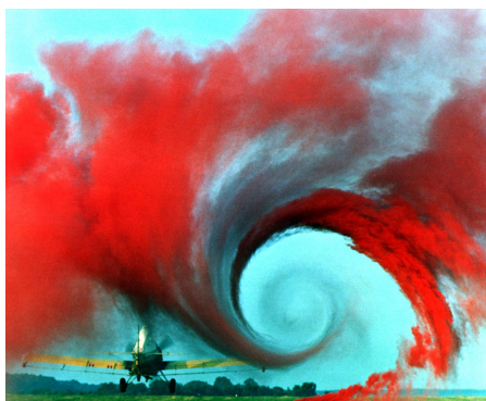
(a) Wake vortex study from NASA Langley Research Center [NAS90]. The unsteady flow around a starting agricultural plane is made visible using smoke injection. A huge pattern of swirling particle motion is created by the aircraft's wake vortex.
