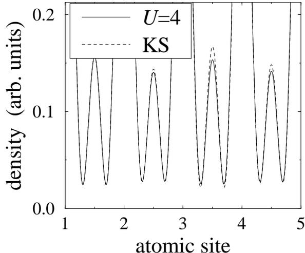
FIG. 1. Electron density of the eight-site Hubbard chain ( $U = 4$ ) together with that of the Kohn-Sham system that reproduces it as closely as possible (KS), visualized by assuming a particular form of orbitals (see the text). There is good agreement at the ends of the chain (site 1), but increasing deviation towards the center (site 5). The deviation illustrates the fact that the density of the interacting system is *not* noninteracting  $v$  representable.
