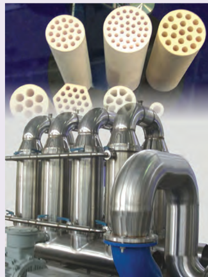
Ceramic filters used at Radford Meats. Image provided by the Department of Innovation, Industry, Science and Research.
