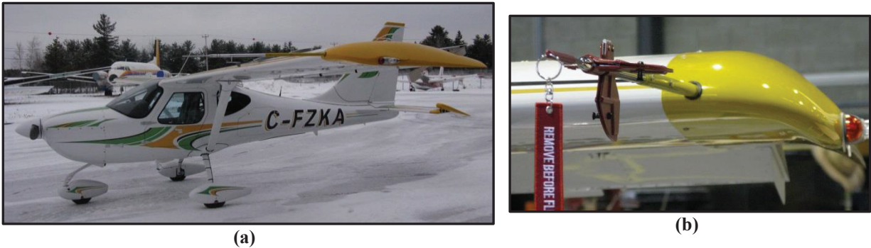
Figure 6.5 : Airdata boom installation on the research aircraft.
