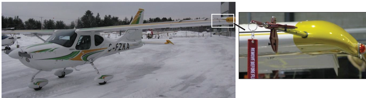
Figure 5.3 : SA160 research platform used for flight testing with close caption on the airdata boom installation. The tests were conducted at Trois-Rivières airport, Québec, Canada.
