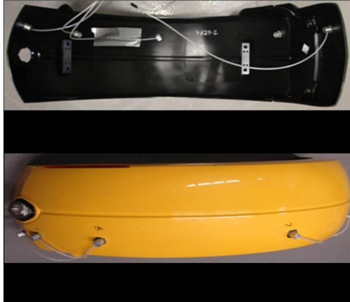
Fig 22: Wheel fender instrumented for wall pressure measurements (a) upper side and (b) lower side
