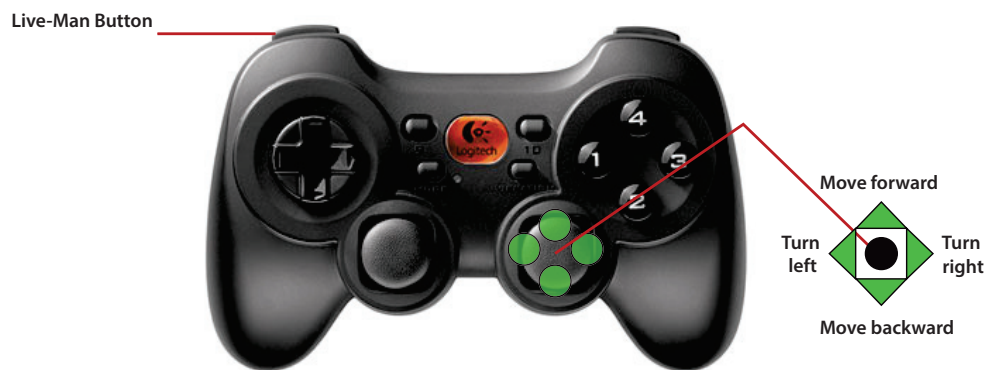
Figure 3.4 Gamepad used to control IRL-1/TR.
