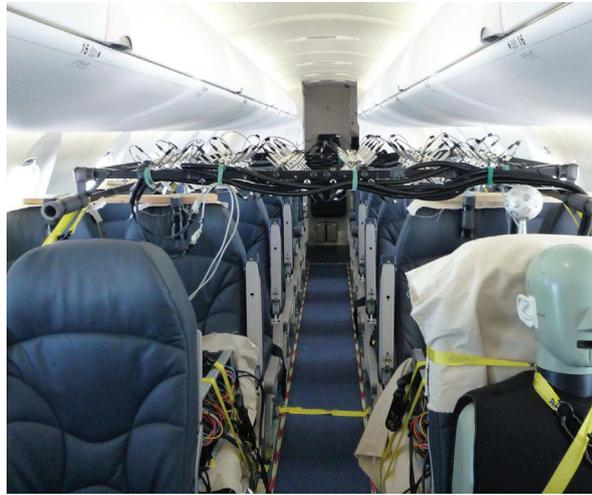
Figure 6.1 Microphone array inside the aircraft cabin for the measurement of the target sound field.
