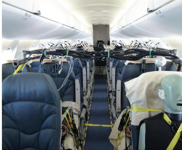
Figure 5.1 Microphone array inside the aircraft cabin for the measurement of the target sound environment.
