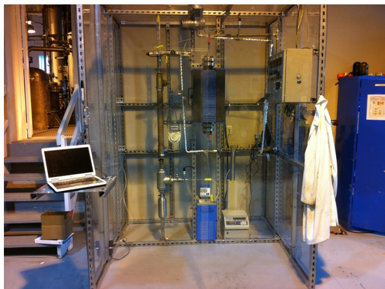
Figure 2.14: Gas flow reactor used for DME carboxylation and DMC decarboxylation
