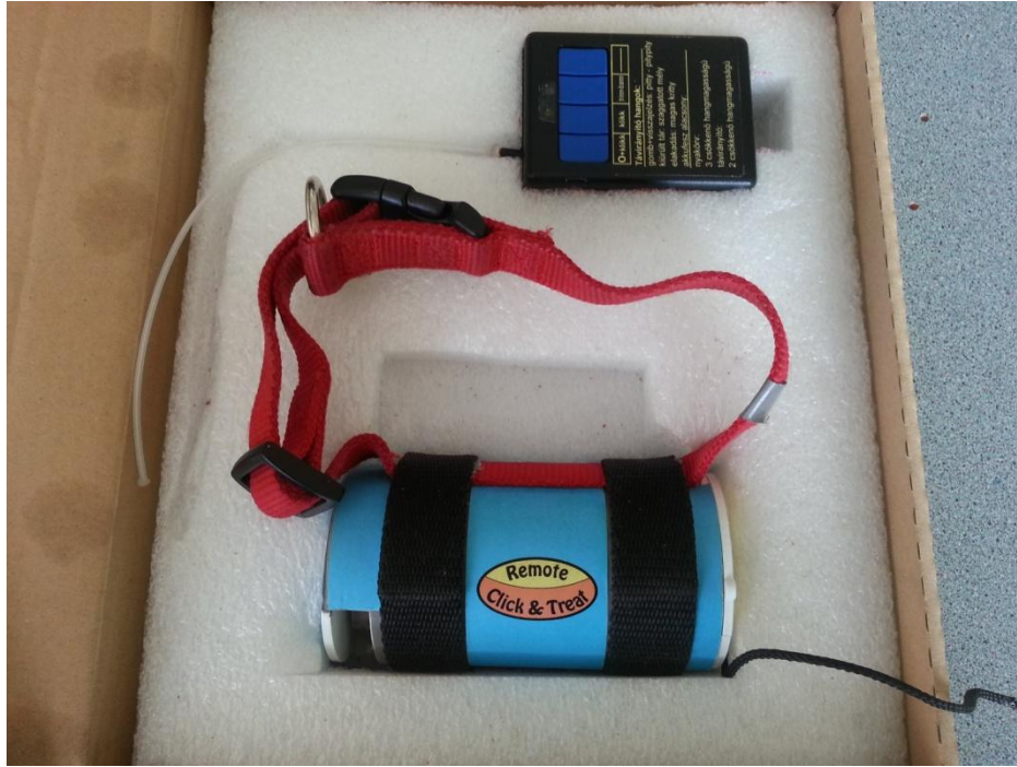
Figure 20. The Click&Treat collar and the controller
