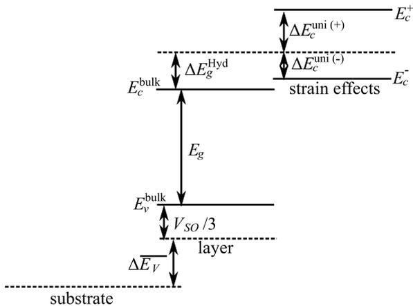
FIG. 1: Energy band schematic (not to scale) for a strained alloy layer on a rigid substrate. To find the potentials of the  $\Delta$  valley minima in the strained layer, the difference in valence band energy and bandgap are calculated before adding the hydrostatic and uniaxial strain effects.
