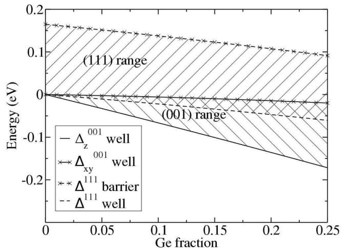
FIG. 2: Usable range of  $\Delta$ -valley offsets for (111) and (001) oriented Si wells with  $\text{Si}_{0.5}\text{Ge}_{0.5}$  barriers as a function of Ge fraction in the substrate. For the (111) orientation the entire quantum well may be used whereas in (001) the  $\Delta_{xy}$  well potential defines the upper limit.
