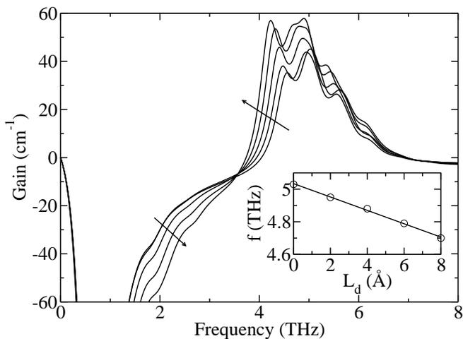
FIG. 5: Active region gain at  $7 \text{ kVcm}^{-1}$ , and 4 K lattice temperature as a function of THz frequency for the design in Fig. 3. Arrows indicate linearly increasing diffusion lengths from 0 to 8 Å. The resulting frequency shift of the largest gain peak is shown inset.
