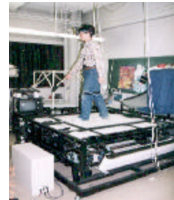
Figure 38 : Tapis roulant 2D (Torus Treadmill)
