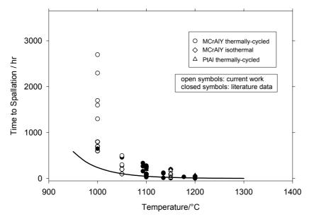
**Figure 4** Experimental data showing the effect of oxidising temperature on the time to TBC spallation for MCrAlY type coatings and for PtAl based TBCs (triangles). The line represents the time at a given temperature to reach a TGO thickness of 3  $\mu$ m, calculated using Eq. 3.
