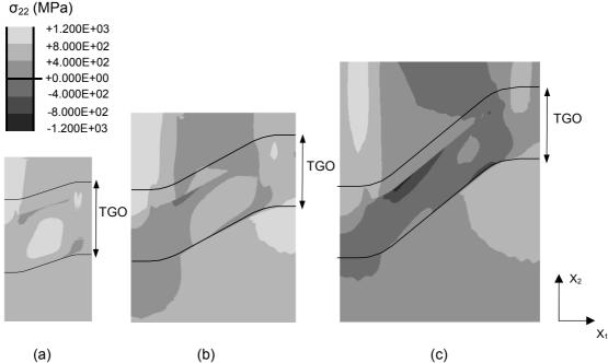
**Figure 6** Three typical out-of-plane stress contour patterns at 25 °C for different geometric parameters with  $\theta_{max}$ = 1000 °C: (a) b =0.79  $\mu$ m, b/a = 0.20, (b) b= 2.47  $\mu$ m, b/a = 0.32 and (c) b = 4.54  $\mu$ m, b/a = 0.48. In all cases, the TGO thickness is 3  $\mu$ m.
