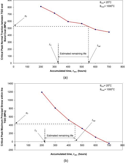
**Figure 13** Illustration of interpolation to obtain TBC failure time,  $t_{\text{fail}}$ , and remaining lifetime for a coating whose failure is controlled by (a) the peak normal traction on the TGO-bond coat interface and (b) peak maximum principal stress within the TGO.
