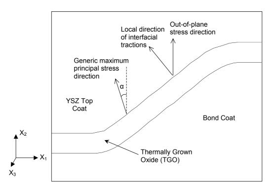
**Figure 2** Diagram illustrating the structure of the TBC system and some of the stresses that are used in determining the failure of the system.
