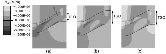
**Figure 7** Contour plots of the out-of-plane stress component  $\sigma_{22}$  after cooling to room temperature from 1000 °C for (a) 61 h, (b) 167 h, and (c) 241 h oxidation. The corresponding TGO thicknesses are 1.91, 2.65 and 3.00 µm, respectively. (Also,  $b = 2.47 \, \mu m$ , b/a = 0.323).
