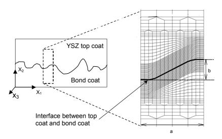
**Figure 5** Illustration of the surface roughness geometric parameters *a* and *b* and a typical finite element mesh of a periodic unit cell used in the modelling.
