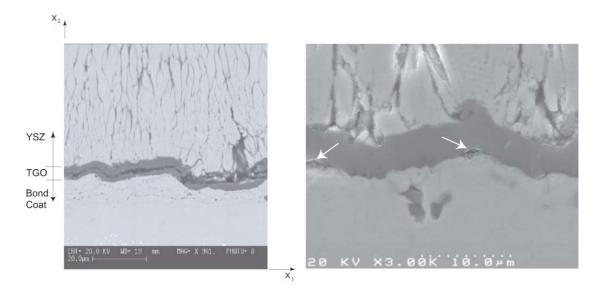
**Figure 1** SEM micrographs showing (a) a typical microstructure of a TBC system (2466 MCrAlY bond coat, EB-PVD YSZ, CMSX4 substrate) after 700 h at 1000 °C, and (b) possible initiation sites (see arrows) of interfacial microcracks between the TGO and the bond coat of a TBC system (bond coat: 2412 MCrAlY, EB-PVD YSZ, substrate: CMSX4) exposed to 1000 °C for 600 h.
