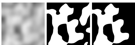
Fig. 14 Object generation with Perlin noise. Left to right: Perlin noise, thresholding, selection of the biggest CC .
