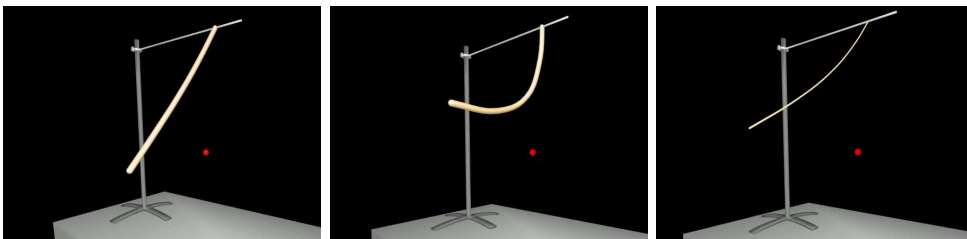
Figure 7: Cantilever beams with several parameters; from top to bottom: ( E = 5e6Pa , D = 0.04m ), ( E = 1e6Pa , D = 0.04m ), ( E = 1e8Pa , D = 0.01m ). Varying diameter and Young Modulus induces different behaviours.
