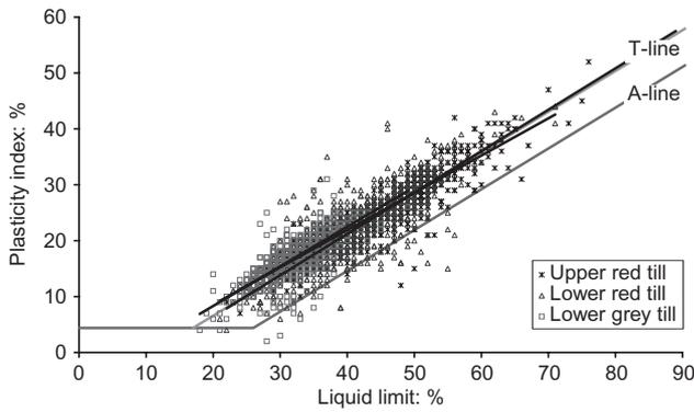
**Fig. 6. Casagrande plot for the tills, showing the relationship between their limits and the T-line, a line parallel to the A-line (the best-fit lines for each till are shown as dashed lines)**
