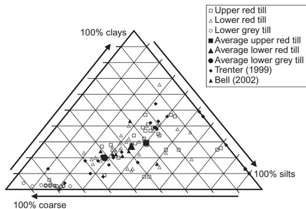
**Fig. 10. Ternary plots for UK glacial tills highlighting variation in the tills according to: (a) fines; (b) clays**
