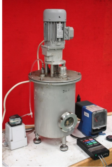
Figure 9.1. Pilot plant digester unit (10 L).
