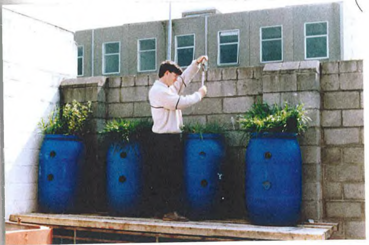
The Four Leaching Containers Used in the Bacterial Survival Experiments
