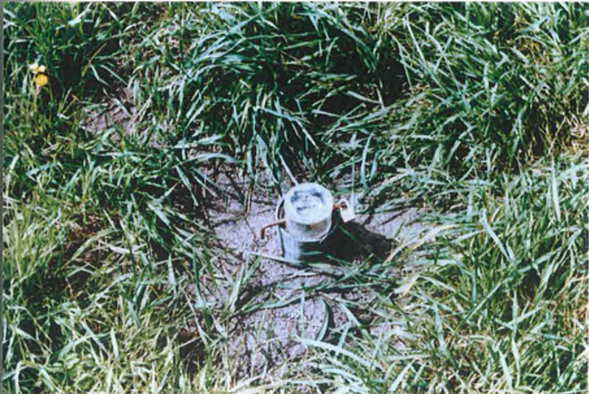
Plate 3.3.2 Monitoring Well - Head Protection
